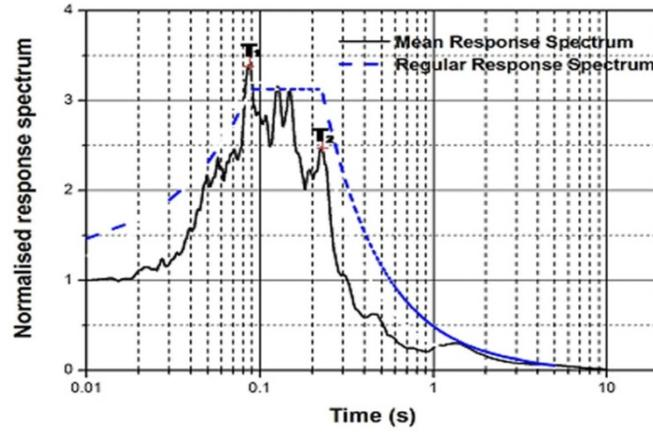
**Figure 3.3.** Normalized elastic response spectrum for 5% damping
