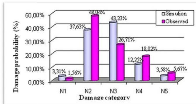
**Figure 3.4.** Histogram of the damages for 3,663 buildings in Boumerdès city: observed (CGS in situ evaluation), and estimated.
