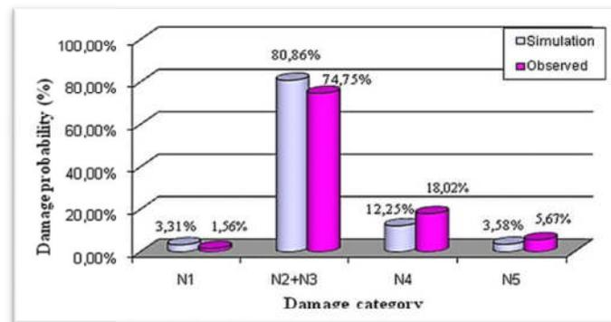
**Figure 3.5.** Comparison of the observed and simulated building damages in Boumerdès city.
