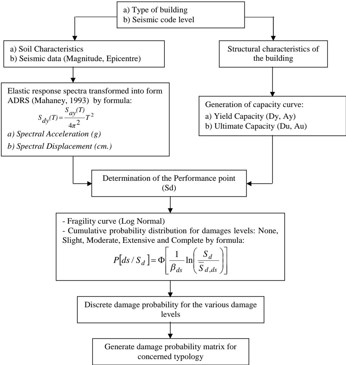
**Figure 2.1.** General flowchart of seismic damage evaluation procedure
