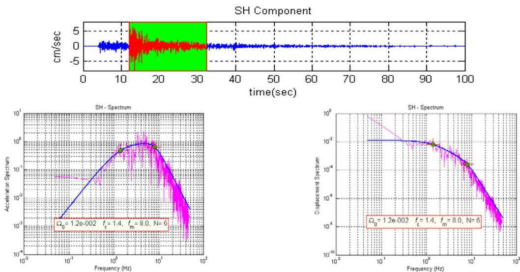
**Figure 2** An example of SH component of velocity time history of earthquake recorded at Vinakhal on short period seismograph. The acceleration and displacement spectra along with fitted source model.
