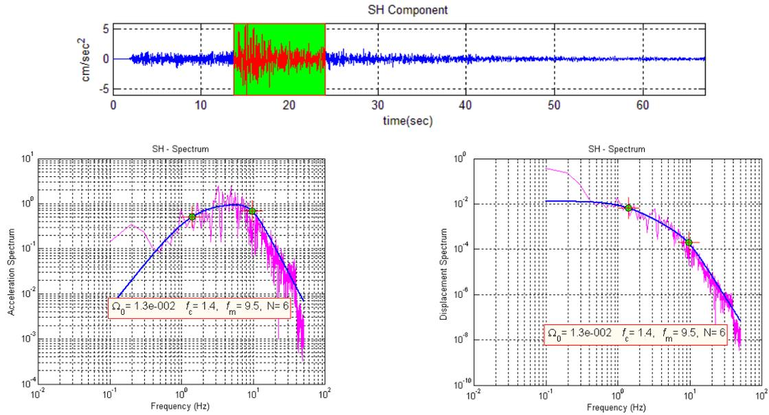
**Figure 3.** An example of SH component of acceleration time history of earthquake recorded at Dhanolti on strong motion instrument. The acceleration and displacement spectra along with fitted source model.
