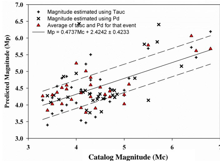
**Figure 5.3.** Plot of Predicted magnitude vs Catalog magnitude. Plus represents magnitude using only  $\tau_c$ , the cross are magnitude estimate using  $P_d$  and the solid red triangle is the average of the  $P_d$  and  $\tau_c$  magnitudes for that event.
