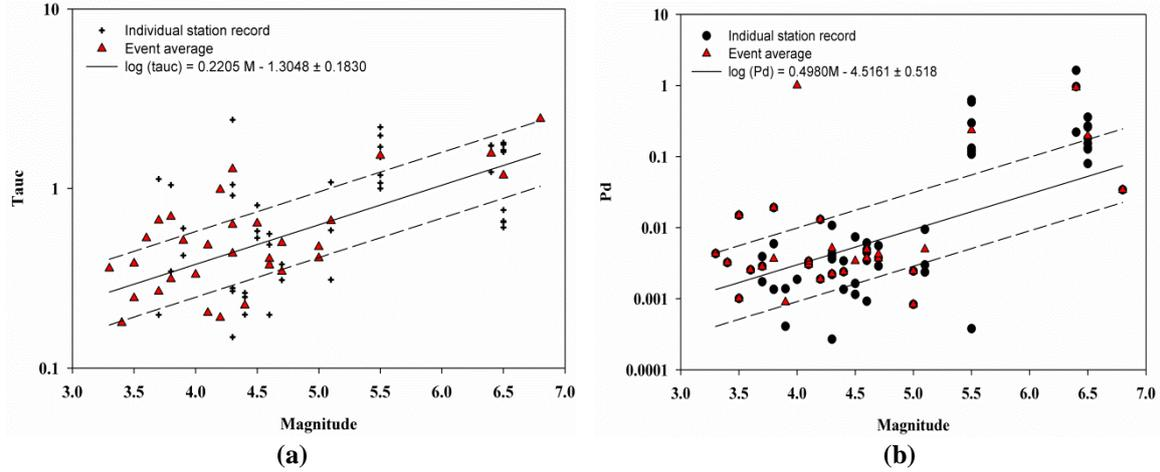
**Figure 5.1.** Plots of regression curve (solid lines). The two dashed lines represent the standard deviation. Plus represents  $\tau_c$  and Pd values at each station and red solid triangle represents average value of  $\tau_c$  and Pd for the event. (a)  $\tau_c$  vs magnitude plot (b) Pd vs magnitude plot for Indian data.
