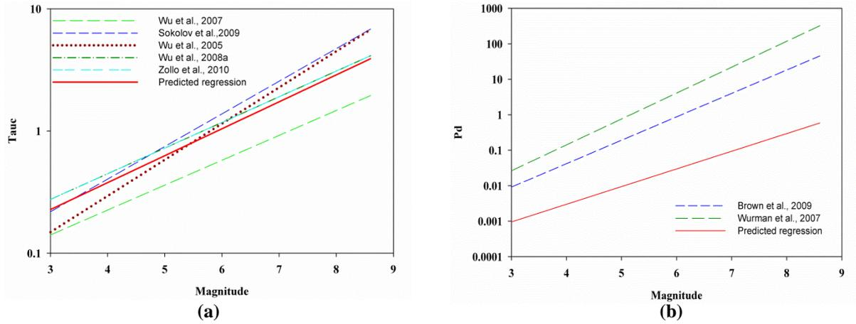
**Figure 5.2.** Comparison of Predicted regression calculated from Indian data with the regressions given by different researchers of the world. Dash and dot lines represent the other researcher's attenuation equation and red solid line represents the predicted attenuation equation. (a)  $\tau_c$  vs magnitude plot (b) Pd vs magnitude plot for comparing goodness of fit of predicted regression.
