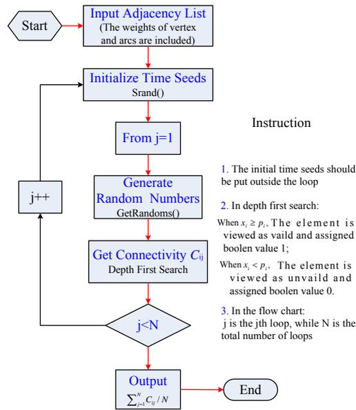
**Figure 4.1.** Flow charts of network reliability analysis based on Monte Carlo method
