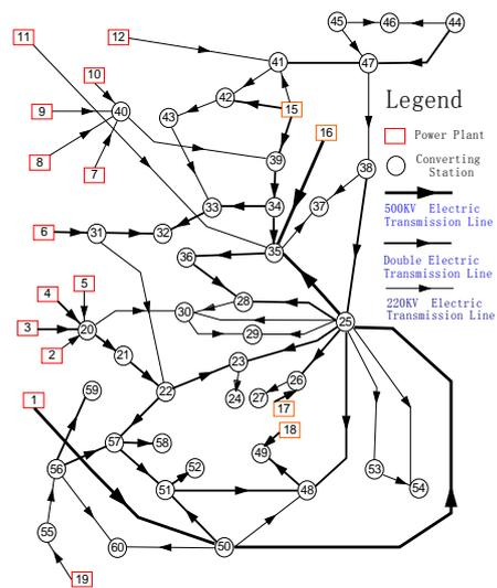
**Figure 5.2.** Basic model of the practical EPS in somewhere
