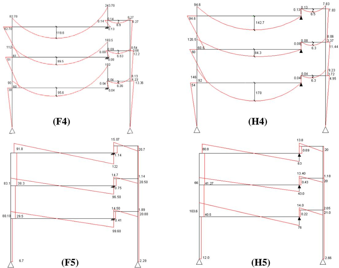
Figure 6. (F4-H4) Moments under lateral load, (F5-H5) Shear forces under lateral load
