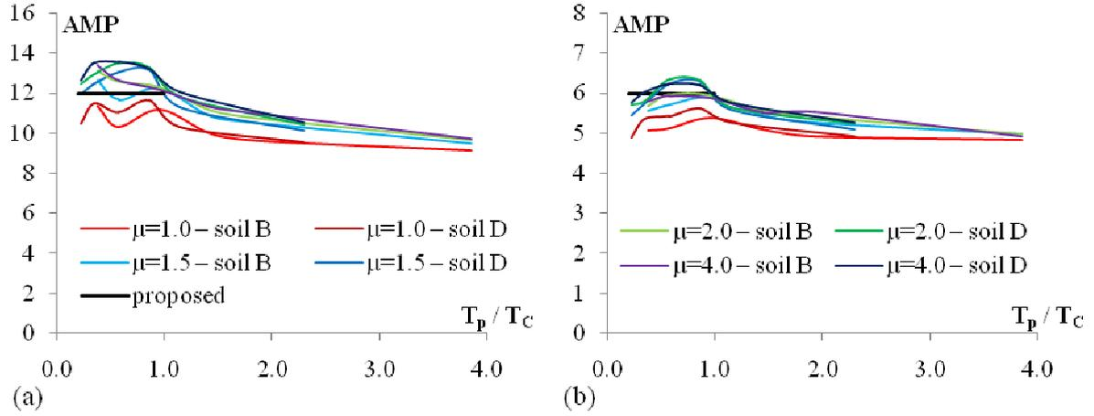
**Figure 5.** Computed and proposed amplification factors AMP in the case of EP model for (a) 1% damping and (b) 5% damping of SS
