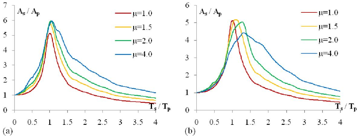
**Figure 4.** Floor response spectra normalized to the peak acceleration of the PS ( $T_p=0.3$  sec) for (a) EP and (b) Q models (soil type B, 5% damping of PS and SS)
