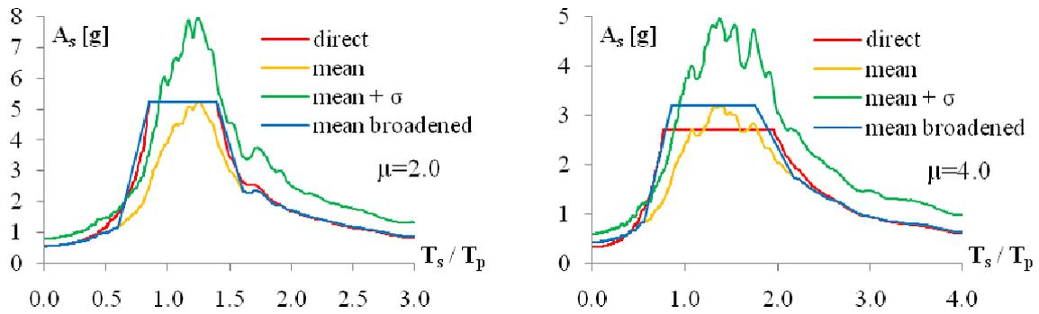
**Figure 8.** Floor response spectra for Q model of PS (soil type B,  $T_p=0.3$  sec, 5% damping of PS and 1% damping of SS)
