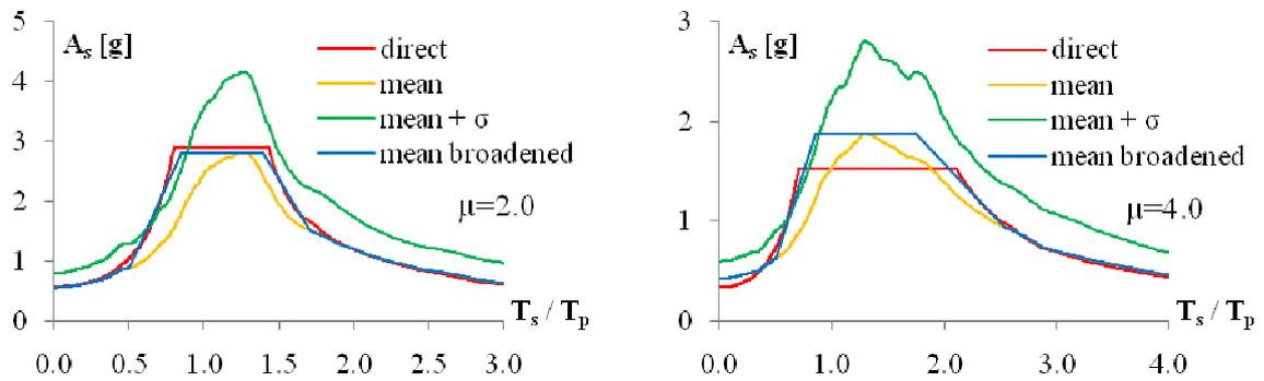
**Figure 12.** Floor response spectra for Q model of PS (soil type B,  $T_p=0.3$  sec, 5% damping of PS and SS)
