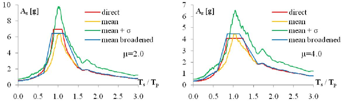
**Figure 7.** Floor response spectra for EP model of PS (soil type B,  $T_p=0.3$  sec, 5% damping of PS and 1% damping of SS)
