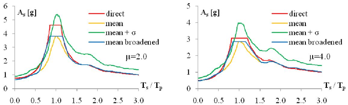
**Figure 13.** Floor response spectra for EP model of PS (soil type D,  $T_p=0.3$  sec, 5% damping of PS and SS)
