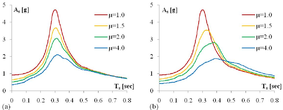
**Figure 2.** Mean values of floor response spectra for  $T_p=0.3$  sec for (a) EP and (b) Q hysteretic models (soil type B, 5% damping of PS and SS)
