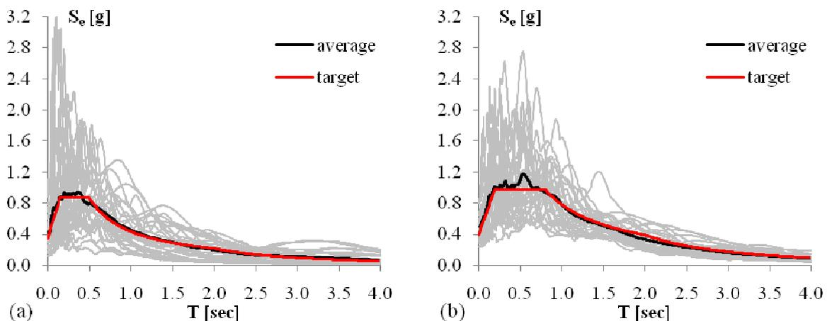
**Figure 1.** Elastic acceleration spectra of individual records, target and average spectrum for the case of (a) soil type B and (b) soil type D (5% damping)
