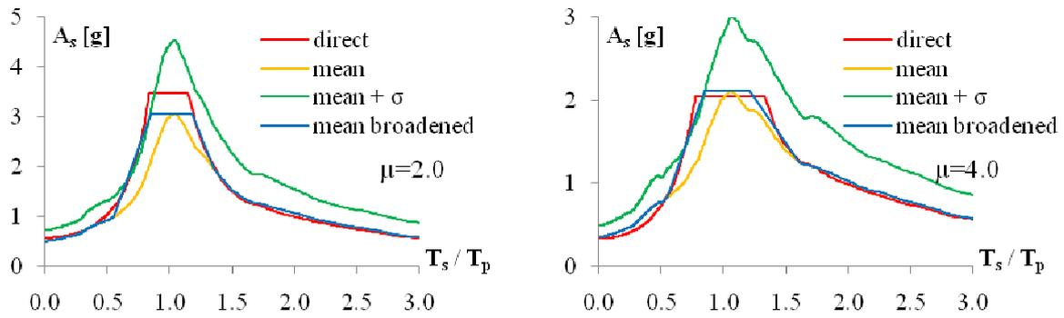
**Figure 11.** Floor response spectra for EP model of PS (soil type B,  $T_p=0.3$  sec, 5% damping of PS and SS)
