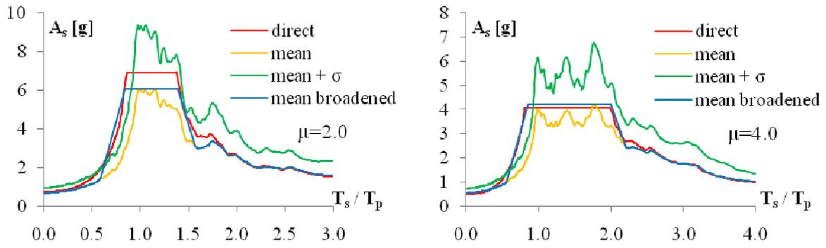
**Figure 10.** Floor response spectra for Q model of PS (soil type D,  $T_p=0.3$  sec, 5% damping of PS and 1% damping of SS)
