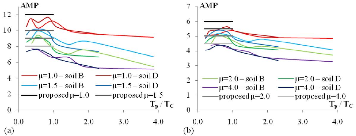
**Figure 6.** Computed and proposed amplification factors AMP in the case of Q model for (a) 1% damping and (b) 5% damping of SS
