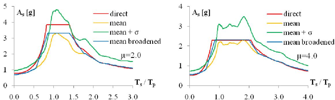
**Figure 14.** Floor response spectra for Q model of PS (soil type D,  $T_p=0.3$  sec, 5% damping of PS and SS)
