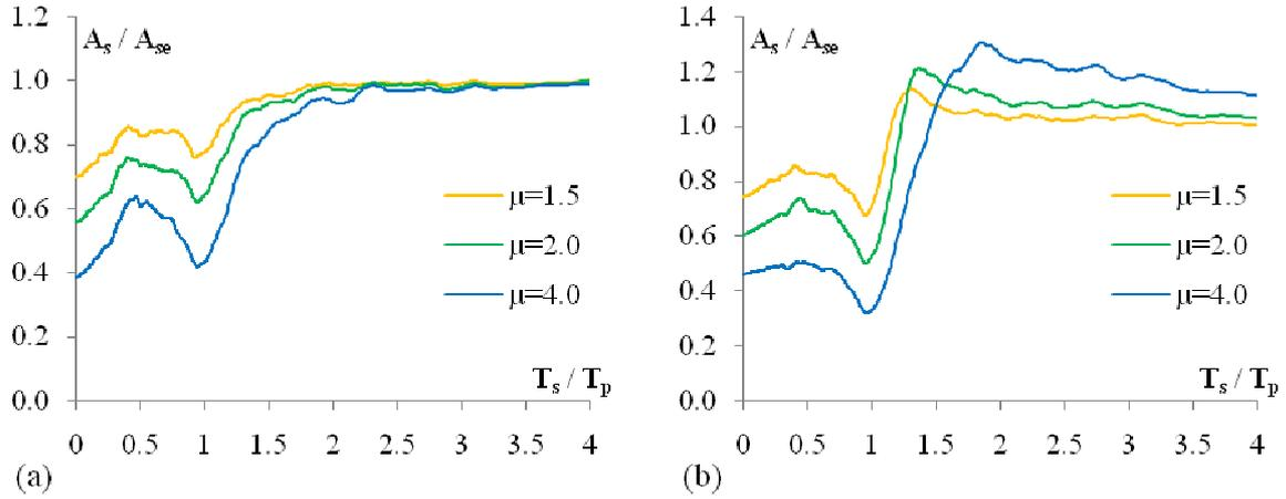
**Figure 3.** The ratio of floor response spectra corresponding to inelastic and elastic PS ( $T_p=0.3$  sec) for (a) EP and (b) Q models (soil type B, 5% damping of PS and SS)
