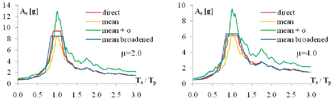
**Figure 9.** Floor response spectra for EP model of PS (soil type D,  $T_p=0.3$  sec, 5% damping of PS and 1% damping of SS)
