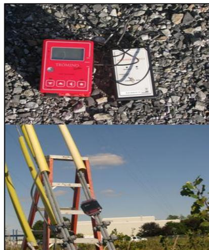
b) Tromograph and radio communication antenna (top) and GP1 accelerometer attached to guy wire (bottom)
