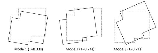
Figure 3.2. Experimentally determined mode shapes
