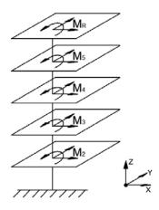
Figure 5.3. Hand calculation model of the Kennedy Library, 3 degrees-of-freedom/floor
