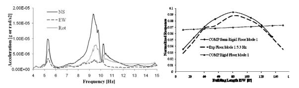
(a) Fast Fourier Transform (b) Mode 1 diaphragm deflected shape **Figure 4.3**. Student experimental shaking results for EWB #5
