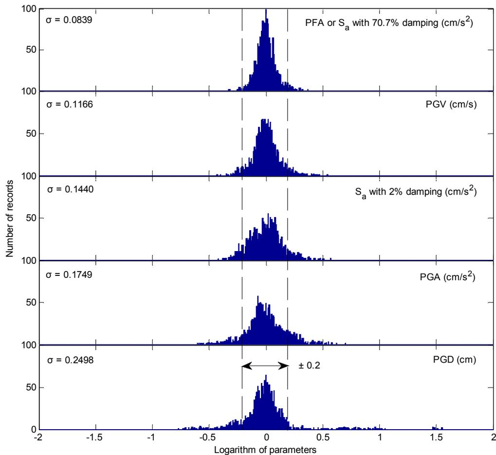
**Figure 5.1.** Comparison of performance of PFA, PGA, PGV, PGD and  $S_a$  in collapse prediction, the intensity measures are normalized by their geometric mean values and plotted in log scale.
