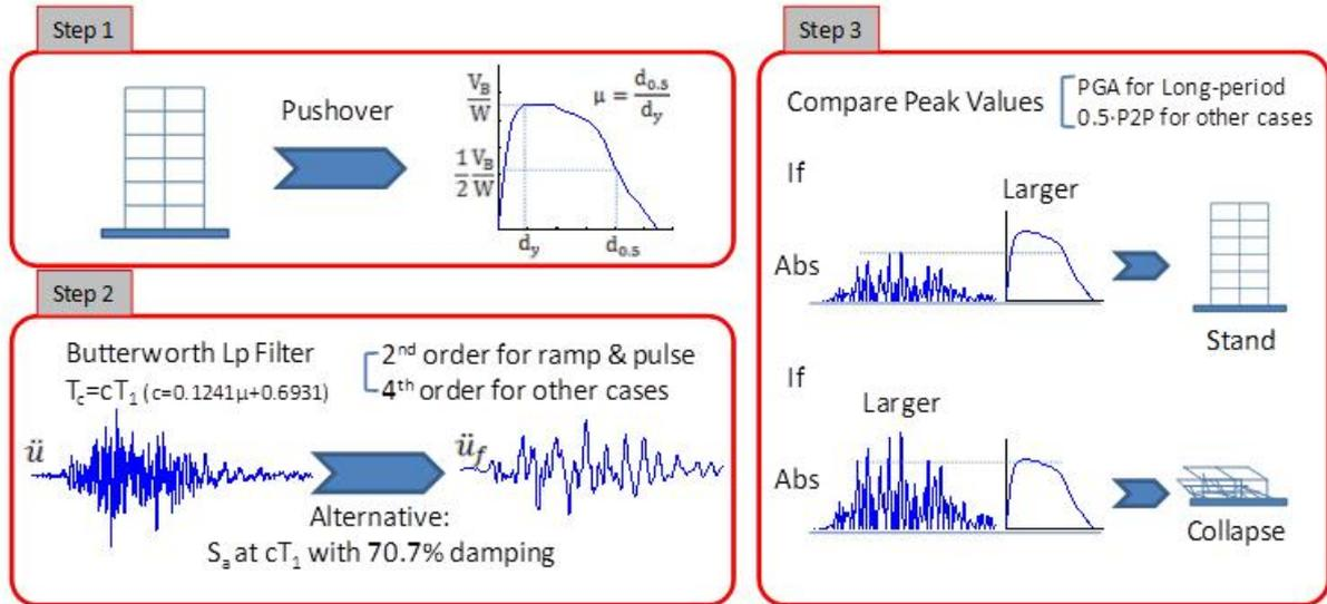
**Figure 1.1.** Procedure of prediction ( $T_1$ -fundamental period,  $T_c$ -cutoff period of Butterworth filter,  $c$ -developed coefficient which depends on the global ductility and ranges between 0.9 and 2.0)
