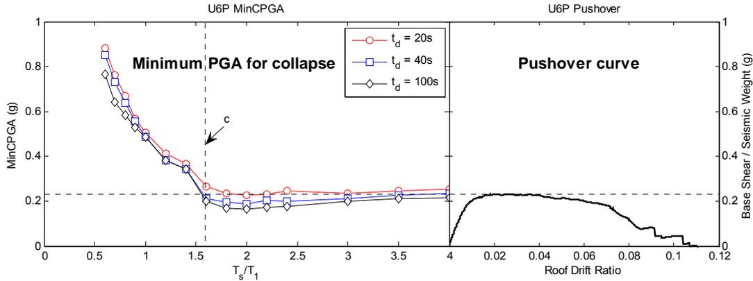
**Figure 2.1.** Example of minimum collapse PGA in sinusoidal ground motions for a US code six-story steel building (U6P) is shown on the left. The pushover curve is shown on the right. A common vertical axis is used for both panels.
