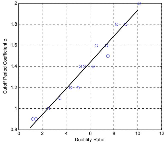
**Figure 3.1.** Regression model of cutoff period coefficient  $c$
