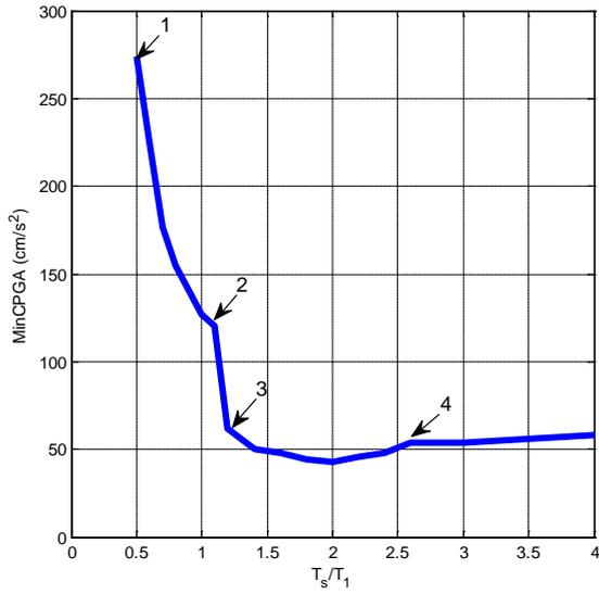
**Figure 1.** Example of minimum collapse PGA for U20B. The motion is sinusoidal with duration of 40s and period  $T_s$ .  $T_1$  is the period of the 1<sup>st</sup> mode, which is 3.47 s for this building.
