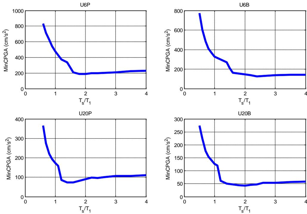
**Figure 3.** Minimum collapse PGA spectra in sinusoidal ground motions for U6P, U6B, U20P and U20B
