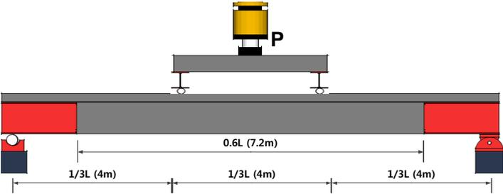
**Figure 8. Test set-up**
