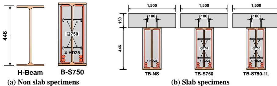
**Figure 7.** Cross section detail of the specimens
