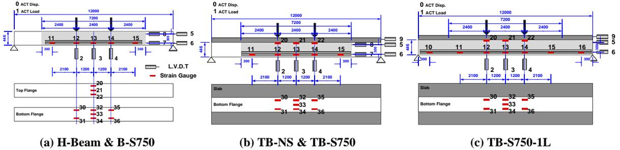
**Figure 9. Measurement of deflections and strains**
