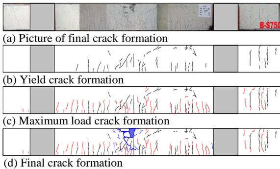
Figure 10. Crack pattern of B-S750
