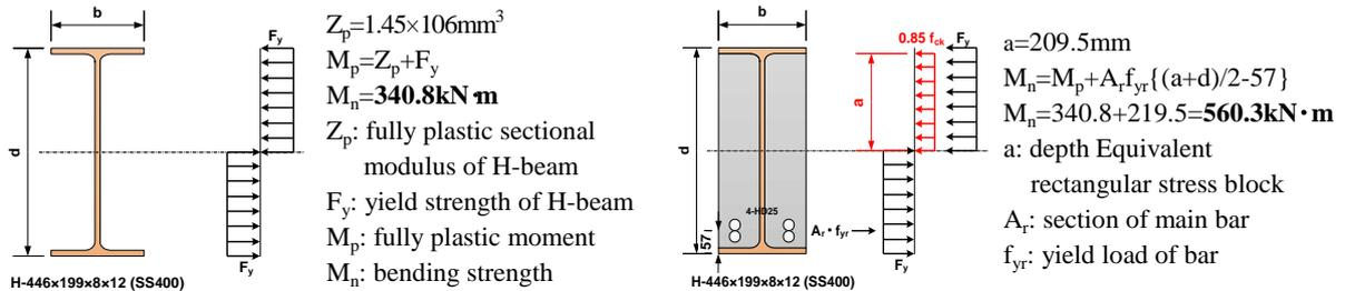
Figure 4. Calculation of the bending strength of H-beam and GSF Beam
