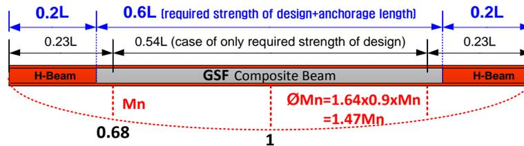
Figure 5. Estimation of placing length
