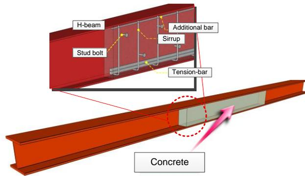
Figure 1. Concept of GSF composite beam
