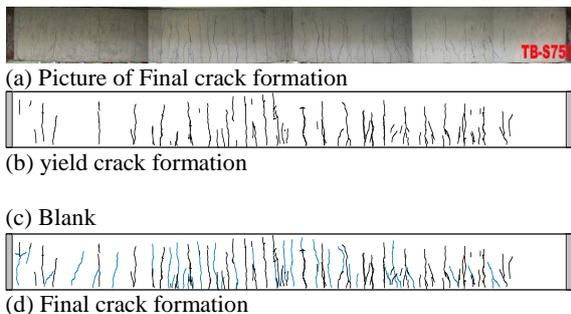
Figure 12. Crack pattern of B-S750
