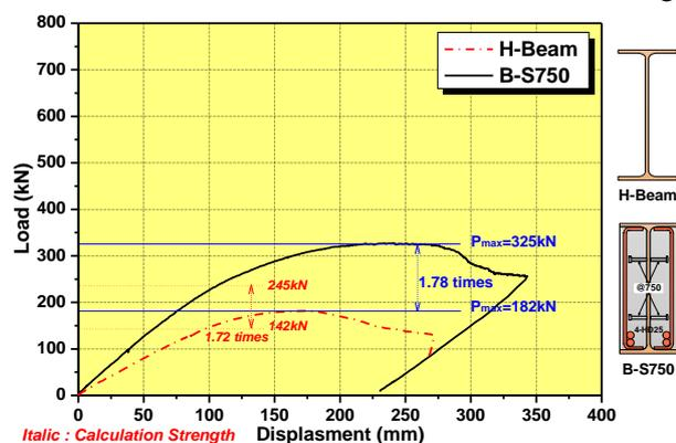
**Figure 16.** Comparison of GSF beam and H-beam
