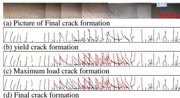
Figure 13. Crack pattern of TB-S750
