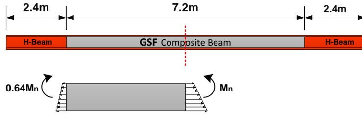
**Figure 6.** Difference between the moment of the center and the end of placing
