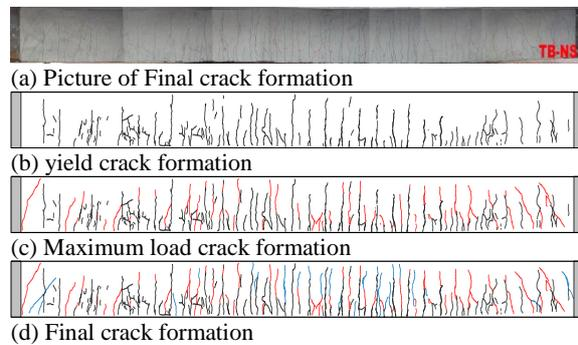
Figure 11. Crack pattern of TB-NS
