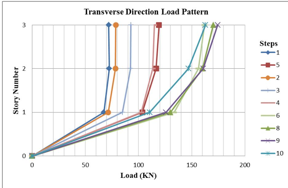
**Figure 2.3.** Transverse direction load pattern.
