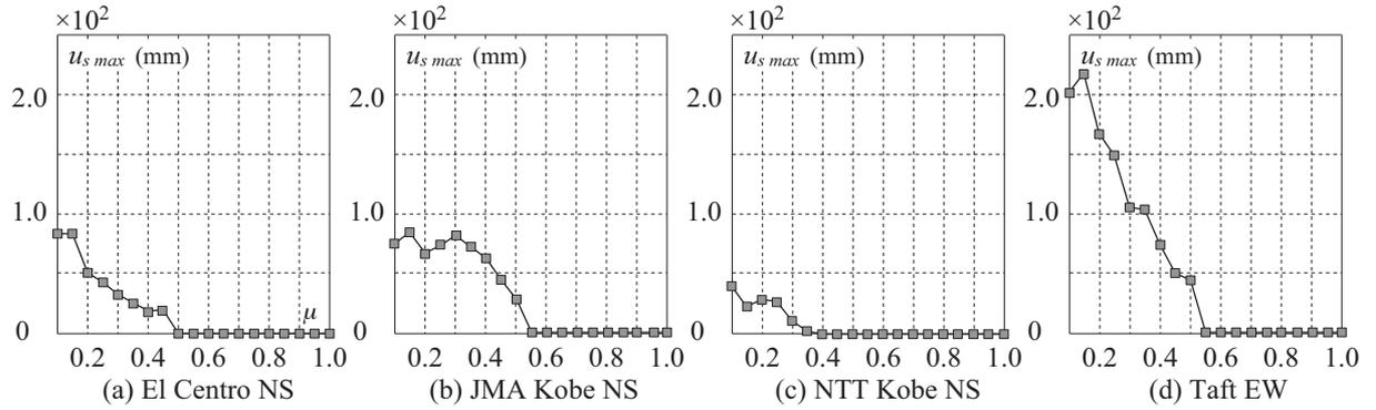
**Figure 5.3.** Maximum sliding displacement of friction elements
