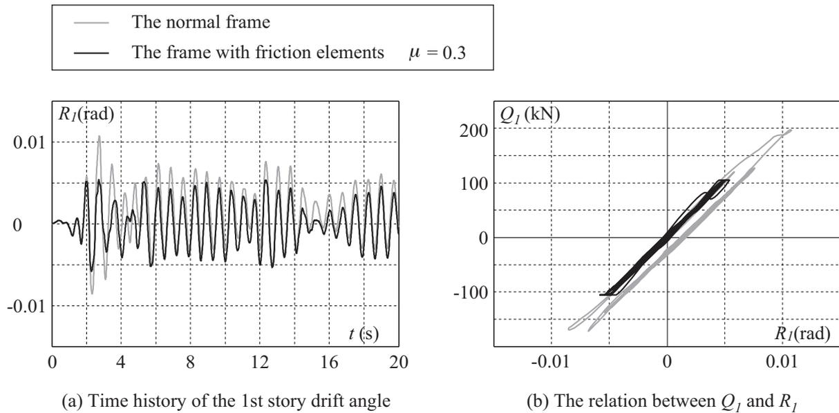
**Figure 4.2.** Dynamic behavior (Sliding coefficient = 0.3)
