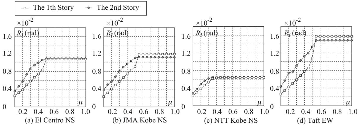
Figure 5.1. Maximum inter-story drift angle
