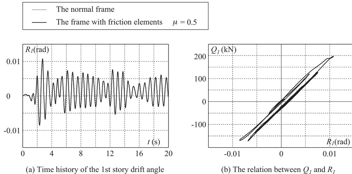
**Figure 4.3.** Dynamic behavior (Sliding coefficient = 0.5)
