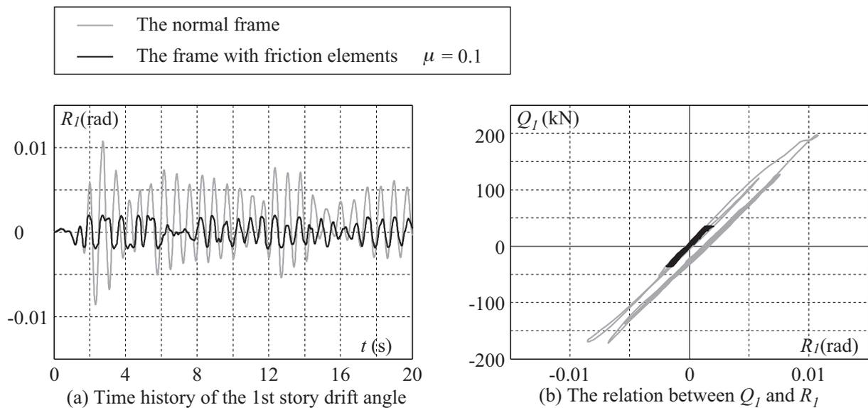
**Figure 4.1.** Dynamic behavior (Sliding coefficient = 0.1)
