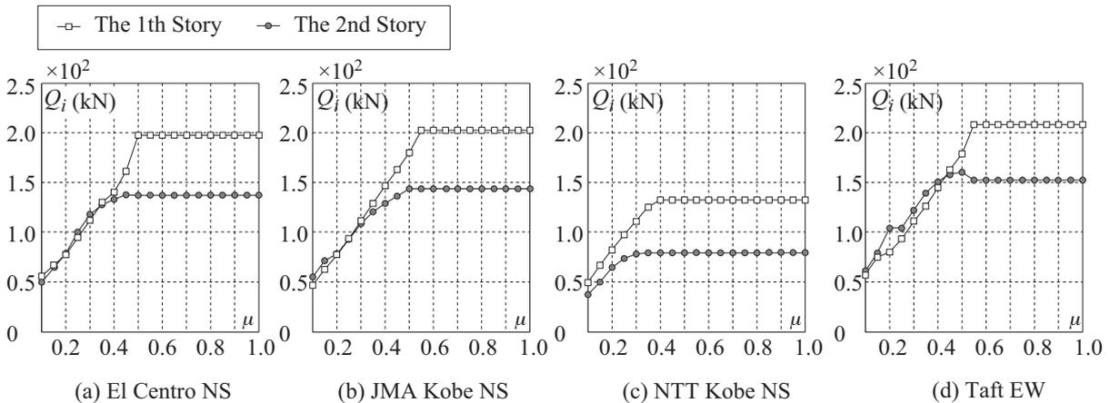
Figure 5.2. Maximum inter-drift shear force
