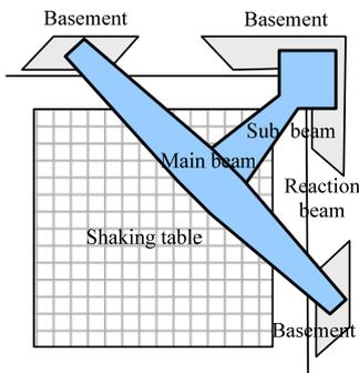
Figure 2.1. Layout of reaction beam
