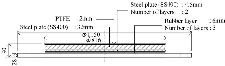
**Figure 4.1.** Sectional view of elastic sliding bearing
