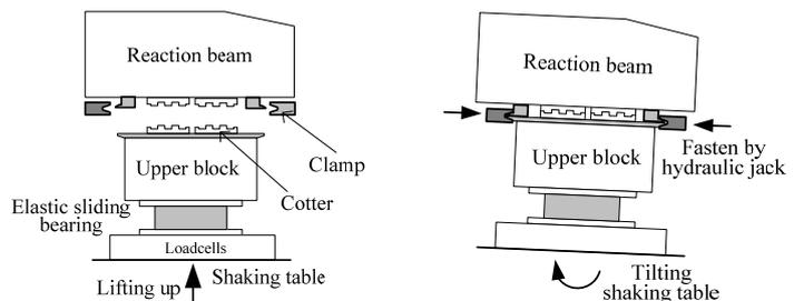
Figure 2.3. Introduction of axial force on the bearing
