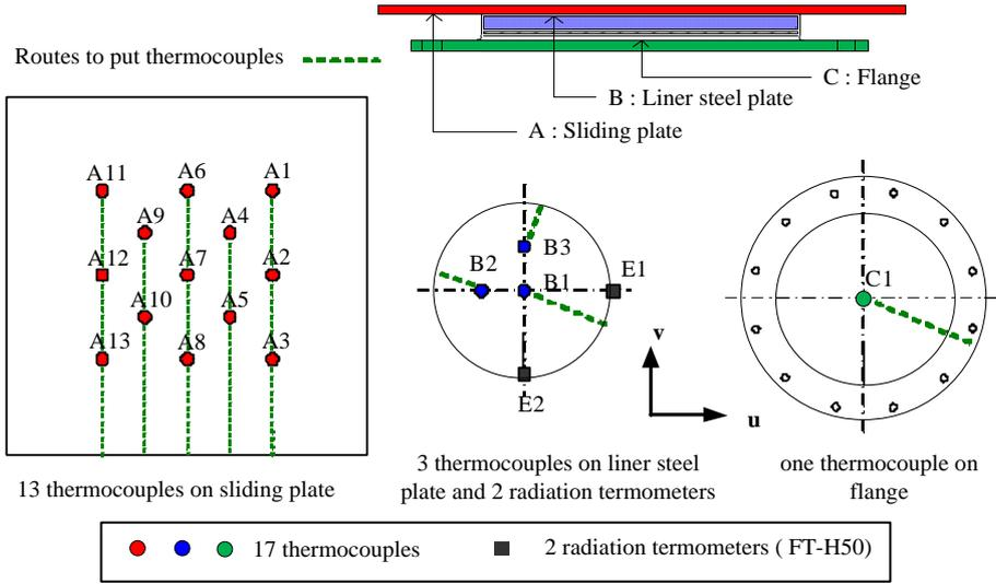
**Figure 4.3.** Layout for temperature measurement
