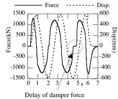
**Figure 5.6.** Damper force and displacement (Case Osv4)
