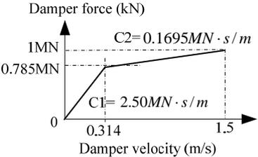
**Figure 5.1.** Damper force characteristics
