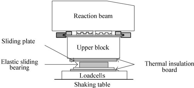
**Figure 4.2.** Experimental set-up for elastic sliding bearing
