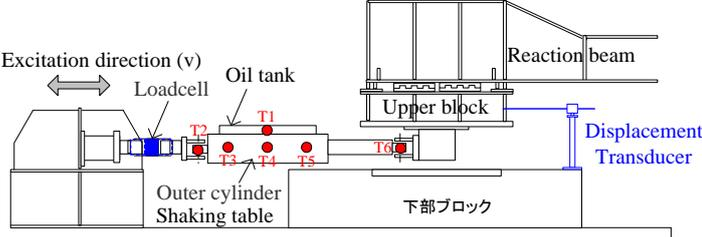
**Figure 5.2.** Layout of measurement sensors
