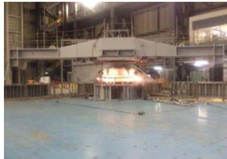
Photo 2.1. Reaction beam in place over shaking table
