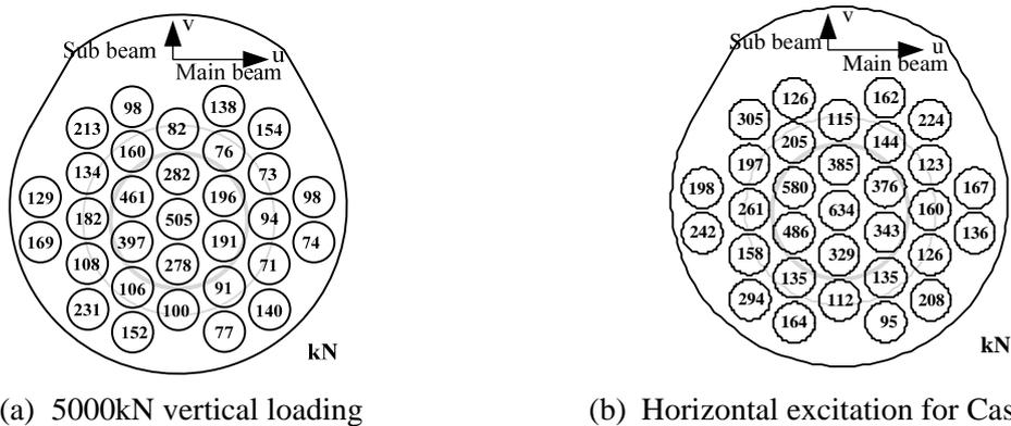
**Figure 3.1.** Maximum vertical loads on 31 load cells
