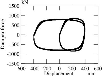
**Figure 5.3.** Damper force and piston displacement for Case Omv
