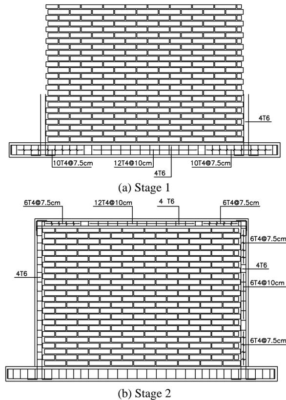
**Figure 2.** Confined masonry wall construction stages
