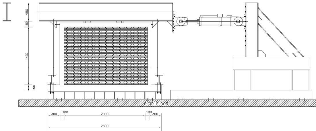
**Figure 4.** Loading setup
