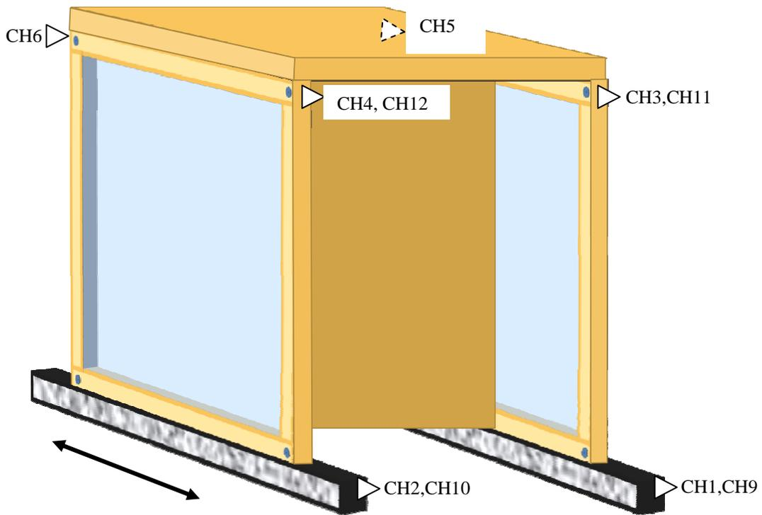
**Figure 3.** Instrumentation of the model with accelerometers and LP's
