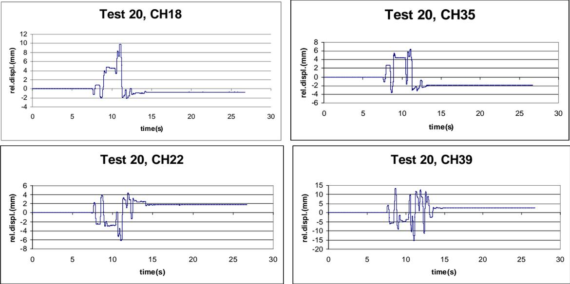
Figure 10. Slipping between the glass and the wooden frame during the Kobe earthquake, test 20
