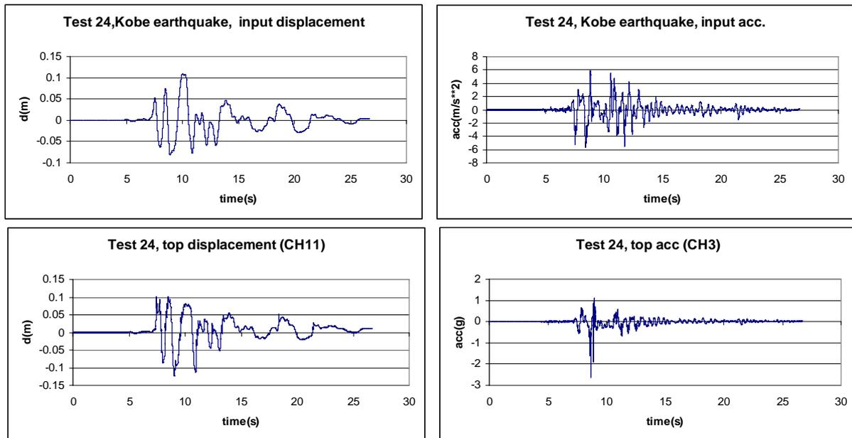
**Figure 8.** Input motion and response of the model, Kobe earthquake, test 24
