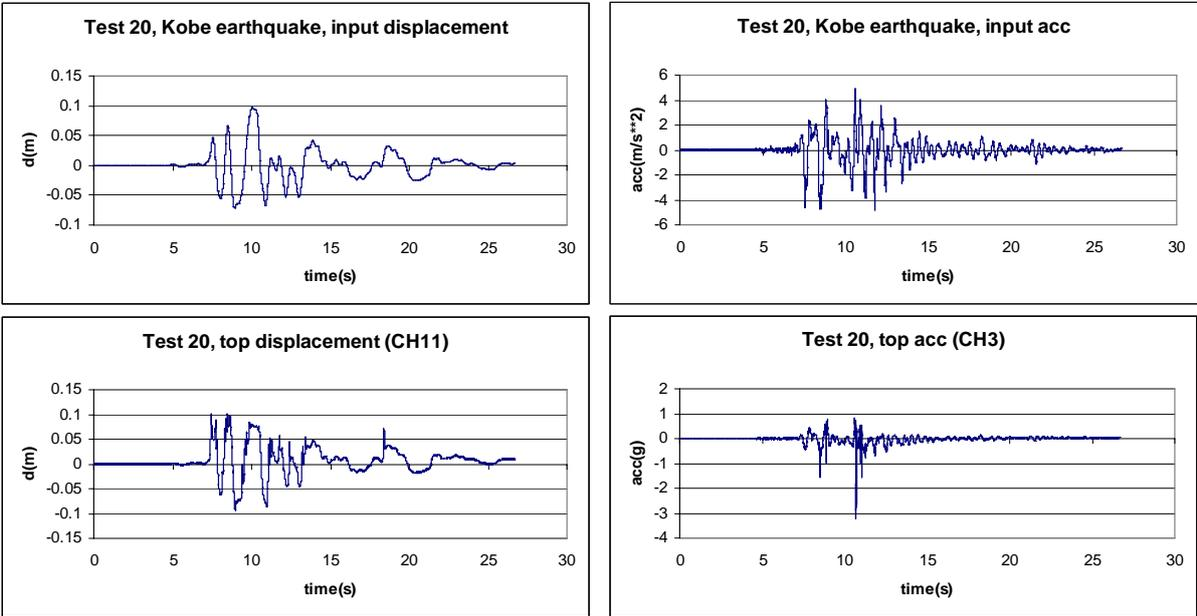
Figure 7. Input motion and response of the model, Kobe earthquake, test 20
