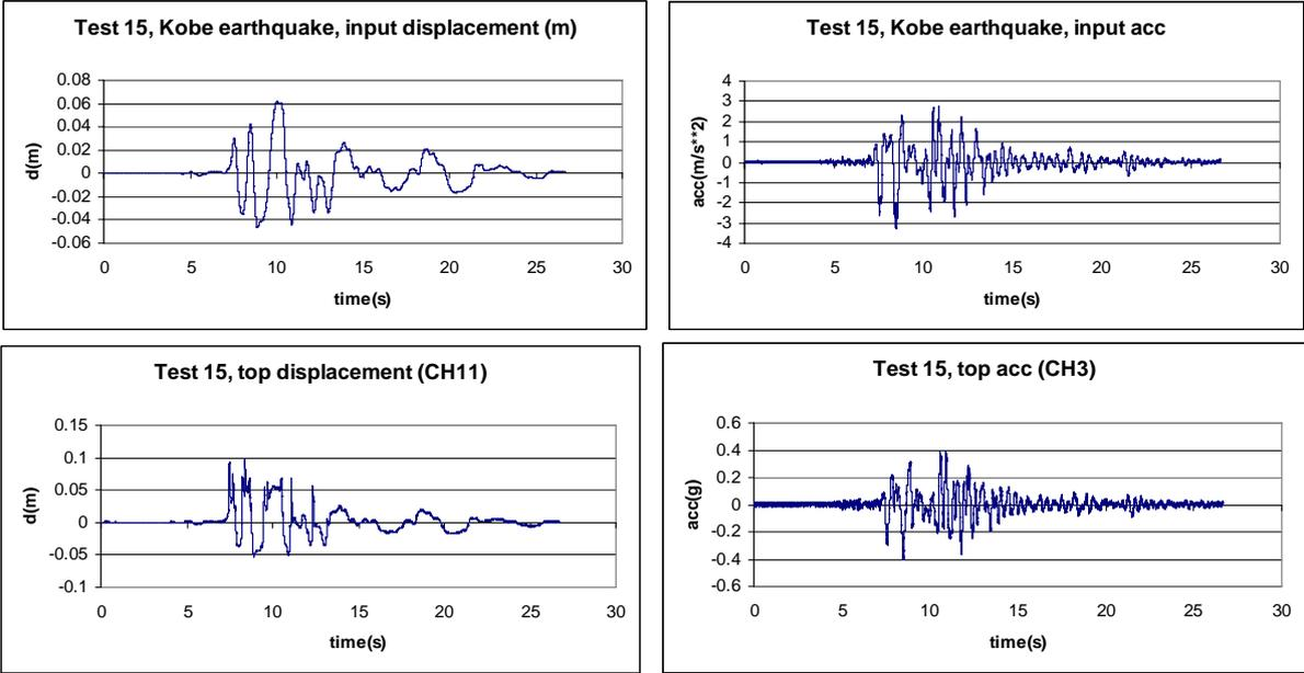
Figure 6. Input motion and response of the model, Kobe earthquake, test 15
