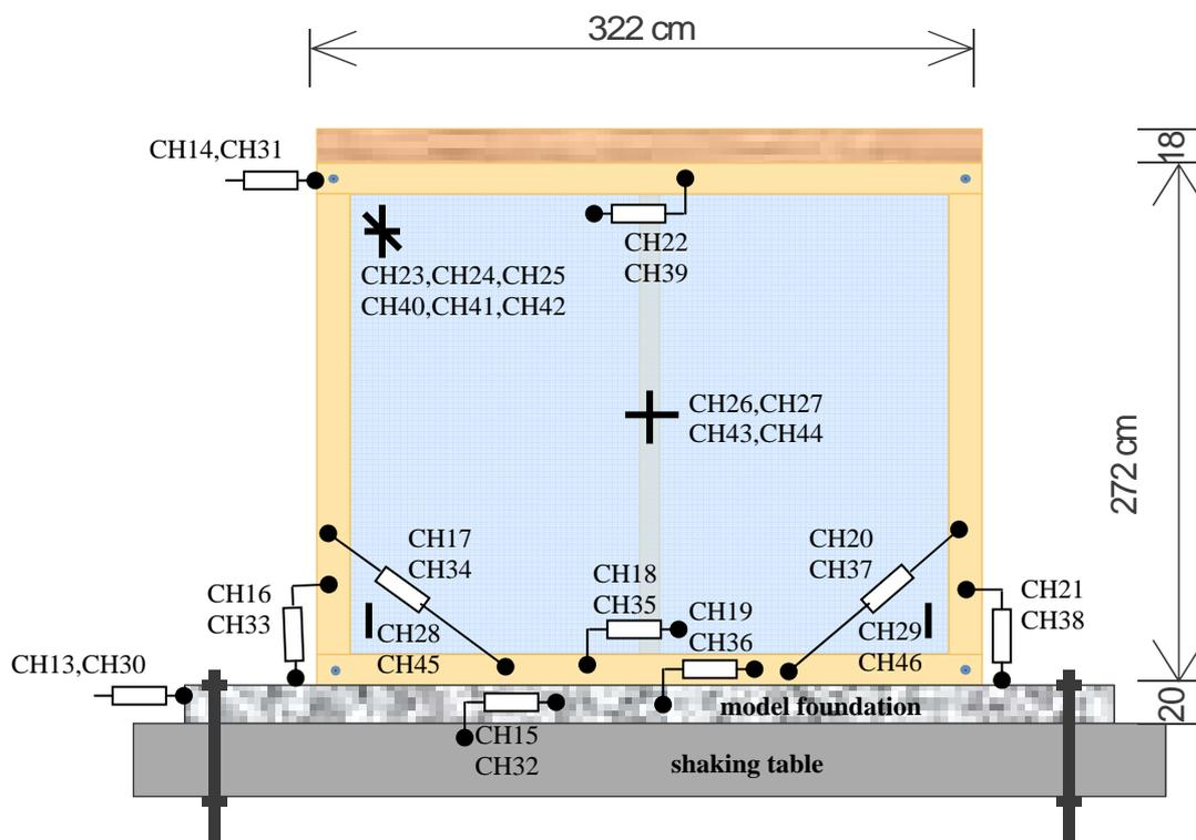
**Figure 4.** Instrumentation of the model with LVDT's and SG (on the glass)
