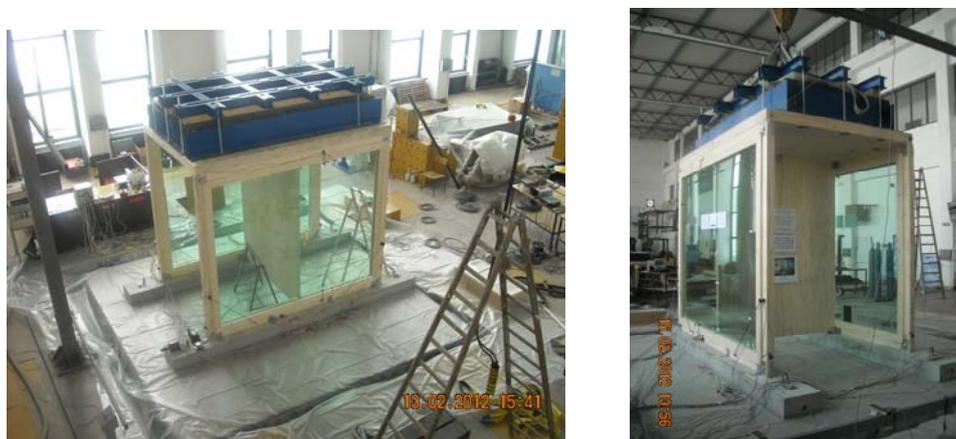
**Figure 2.** Loaded and instrumented model ready for testing
