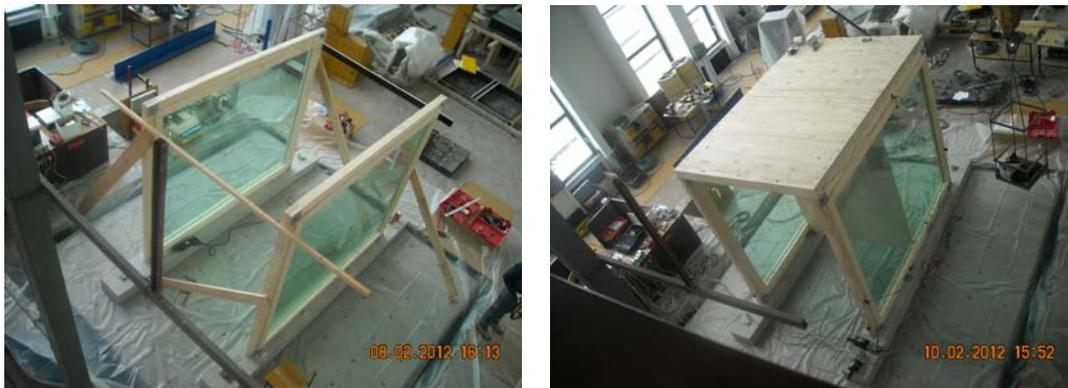
**Figure 1.** Model assembling - fixing of the two composite panels (left), completed model (right)
