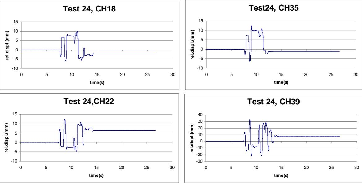
Figure 11. Slipping between the glass and the wooden frame during the Kobe earthquake, test 24
