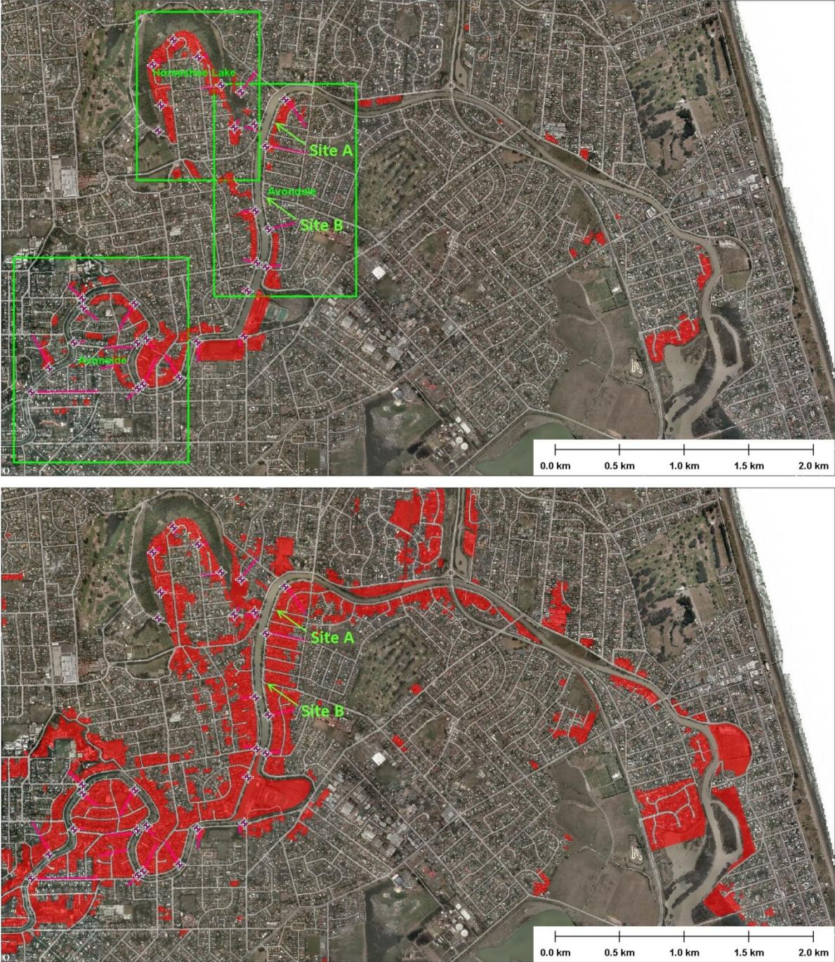
**Figure 2** - Map of eastern Christchurch indicating the extent of liquefaction induced lateral spreading: (a) 4 September 2010 earthquake, with detail locations in Figure 5; (b) 22 February 2011 earthquake
