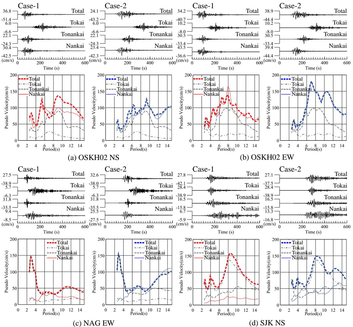
**Figure 3.3.** Calculated velocity and pseudo velocity response spectra
