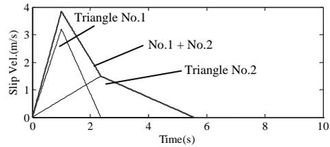
**Figure 2.6.** Example of source time function
