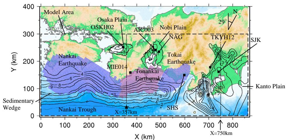
**Figure 2.1.** Model area for FEM calculation and rupture area of Tokai, Tonankai and Nankai earthquake
