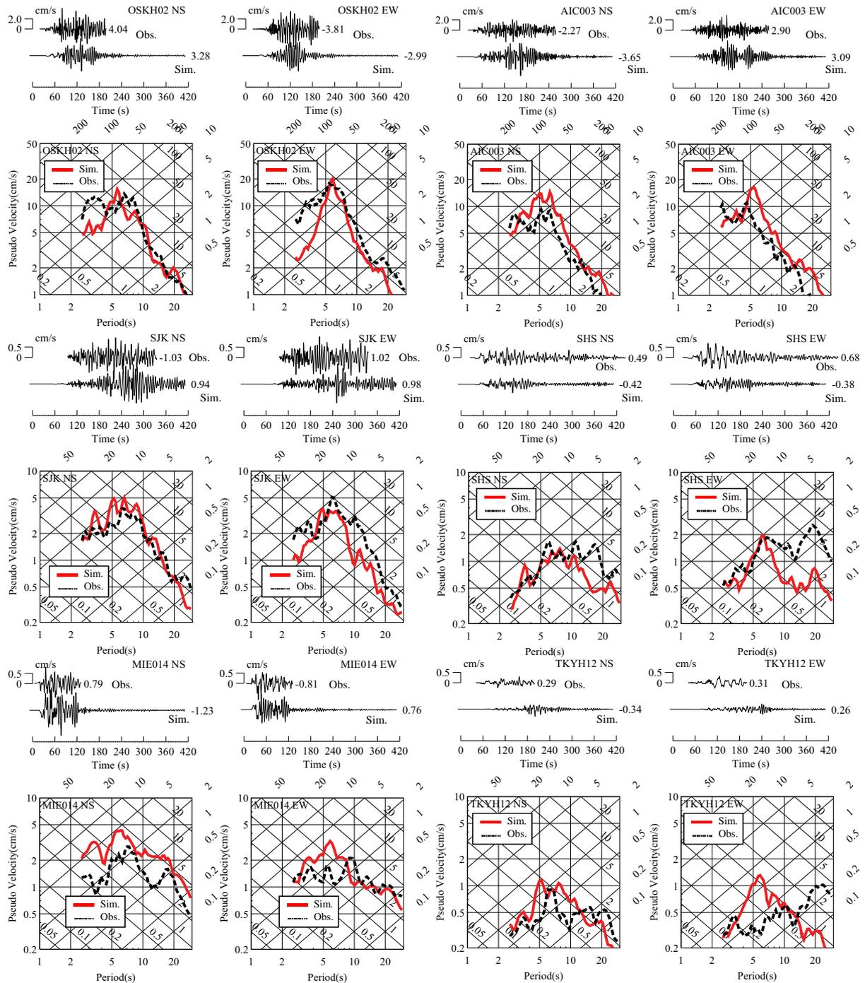
**Figure 2.4.** Comparison of velocity waveforms and response spectra
