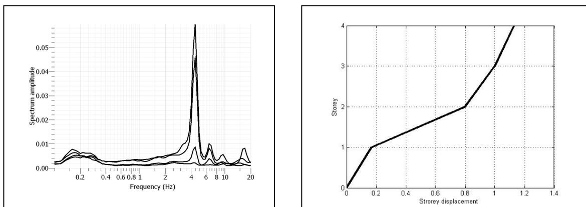
**Figure 6.2:** spectrum amplitude (a), modal shape (b) of the strengthened structure
