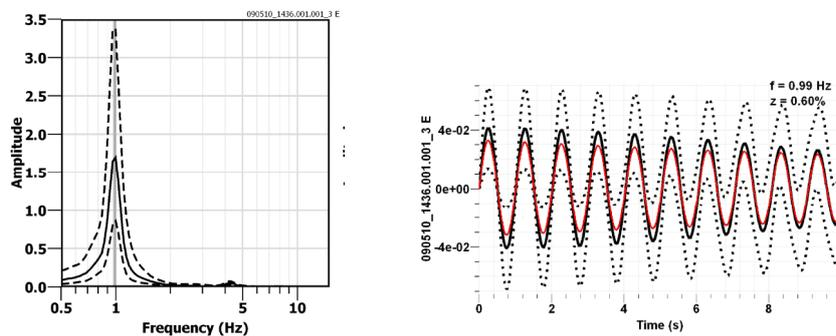
**Figure 4.1.** Frequency and damping of the house before strengthening
