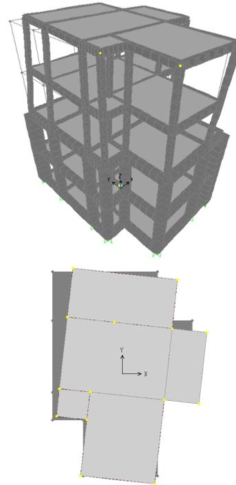
**Figure 7.2:** 1<sup>st</sup> vibration mode (torsion) of the strengthened structure
