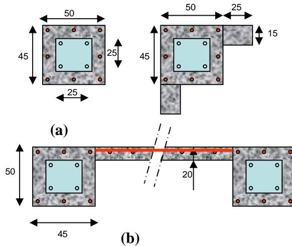
**Figure 2.2:** details of jacketing: (a) column jackets, (b) beam jackets and new slab
