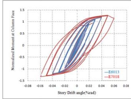
**Figure3.4.** Plots of cyclic response of specimen RC1
