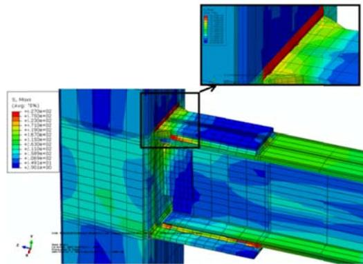
**Figure 3.2.**The von Mises stress distribution in specimen RC1
