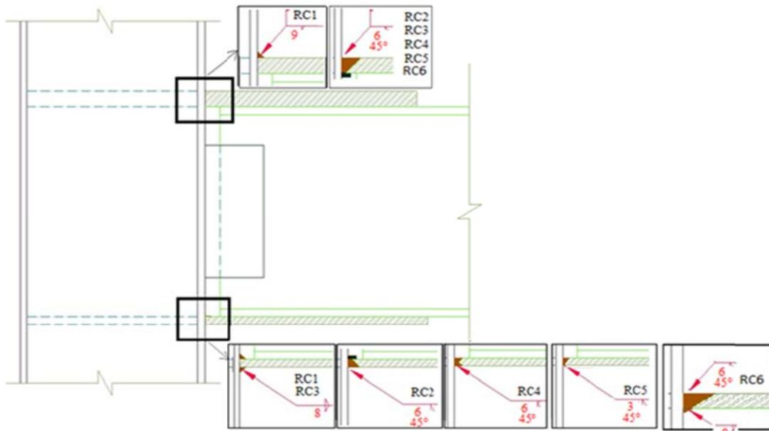
**Figure 3.1.** Geometry and weld types employed to join the flange plate to column
