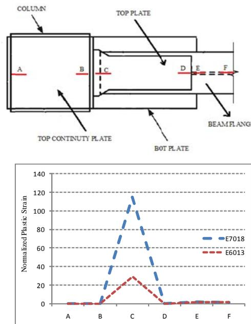
**Figure 3.3.**Strain response for specimen RC1
