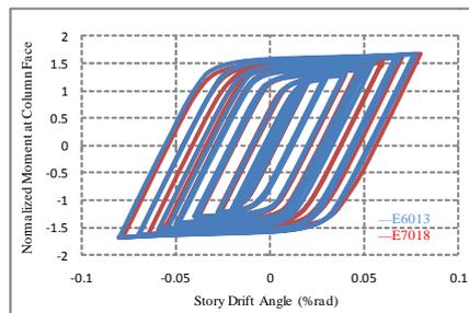
**Figure3.6.** Plots of cyclic response of specimen RC2
