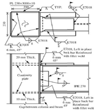
**Figure 2.1.**Detail of experimental specimen
