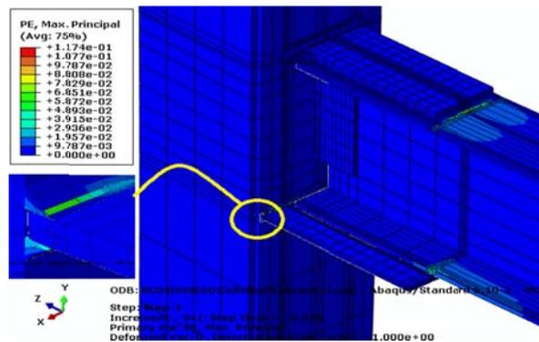
Figure 3.8. The plastic strain distribution in specimen RC3
