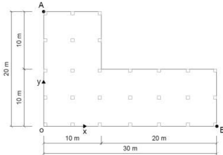
**Figure 3.1.** Schematic representation of the generic plan of the irregular building.
