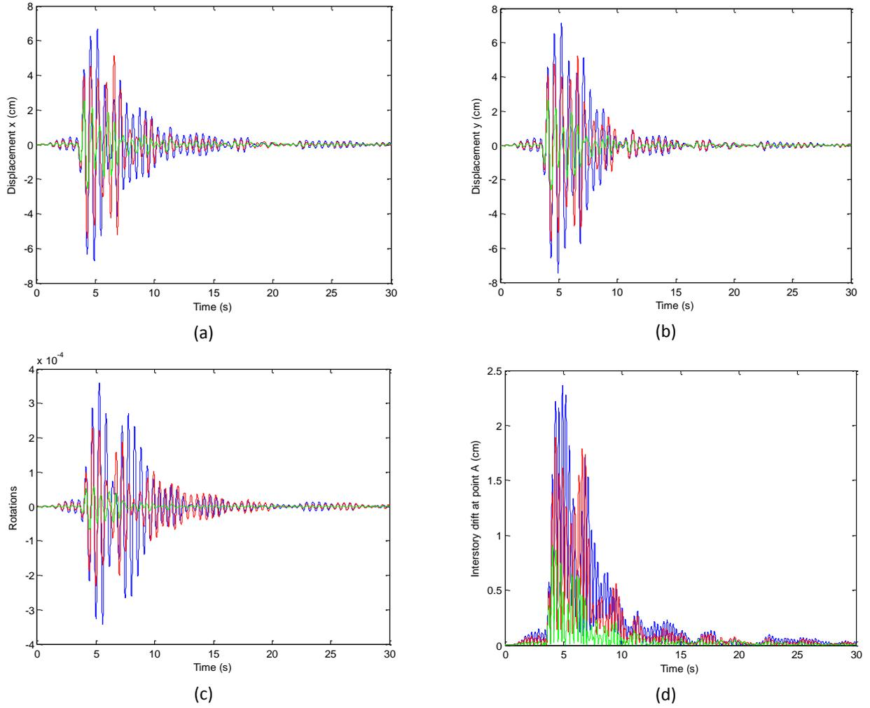
**Figure 3.3.** Time history of the displacements of the elastic center at the top of the structure no.1 along  $x$  (a),  $y$  (b) and rotations (c) and time history of the interstory drift of point A at the top of the building obtained for the uncontrolled, passively controlled and hybridly controlled systems.
