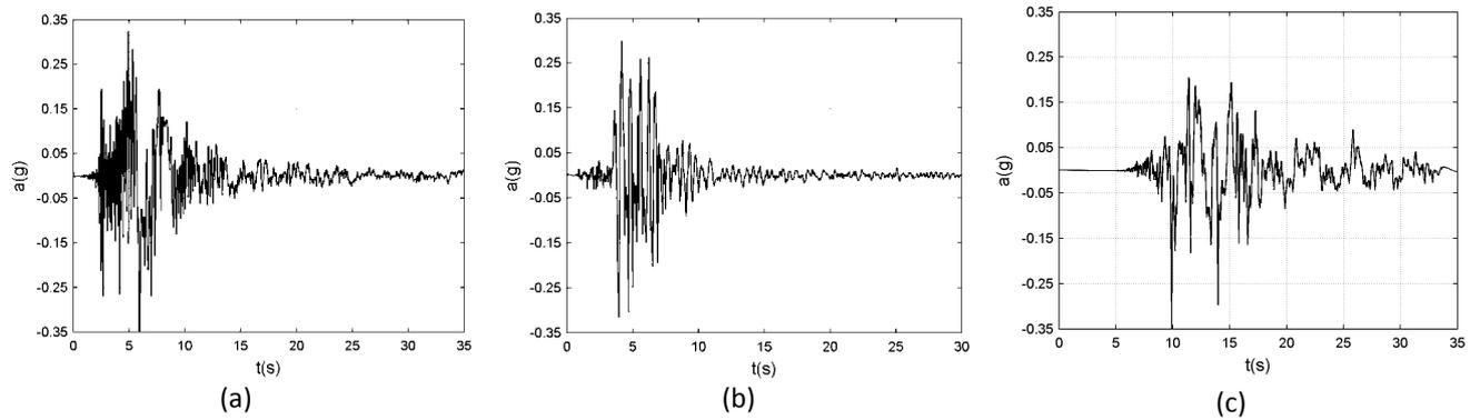
**Figure 3.2.** Accelerograms used for the analyses: Friuli (a); El Centro (b); Kokaeli (c).
