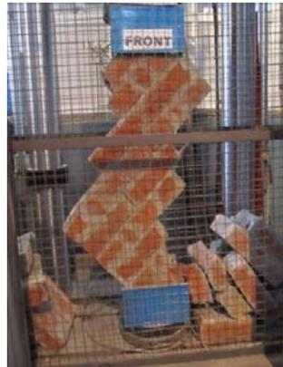
(b) URM two - wythe thick masonry panel
