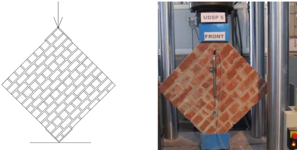
**Figure 2.2** Standard test set up for the diagonal compression test
