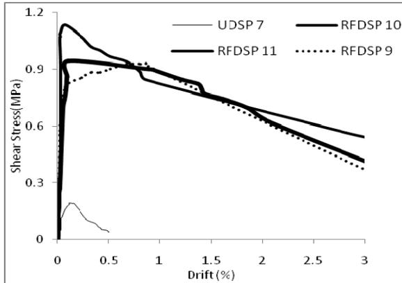
(c) Response of URM and unidirectionally retrofitted two - wythe thick masonry panel
