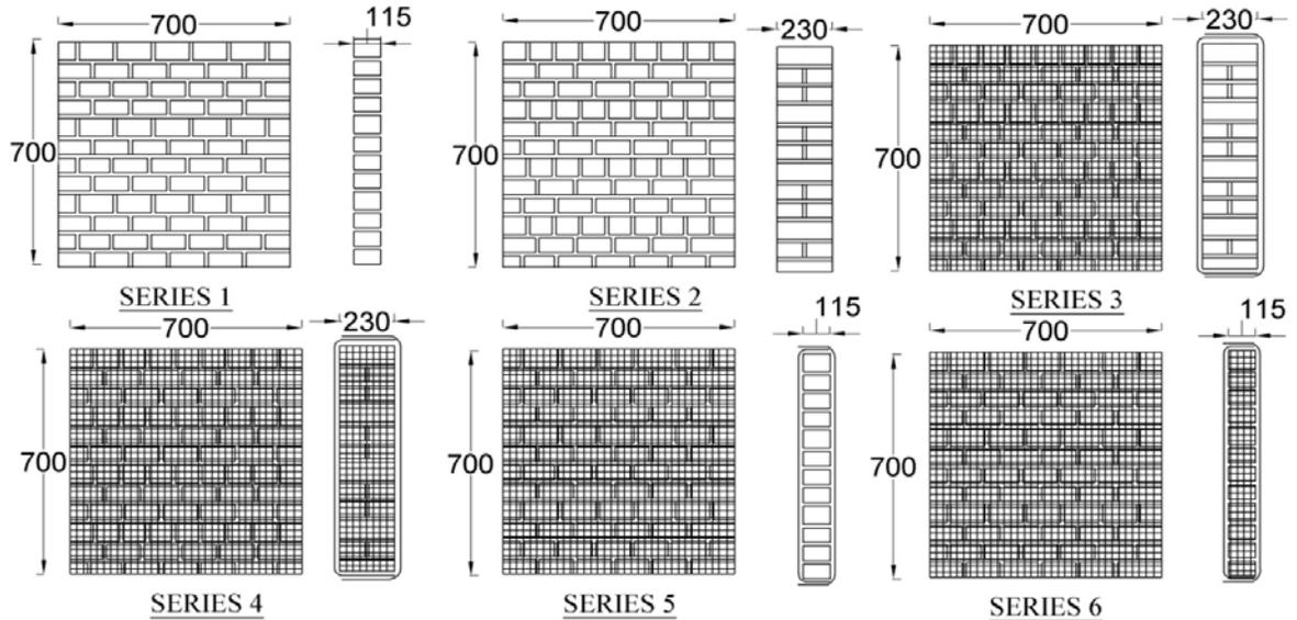
**Figure 2.1** Specimen geometry and retrofit details
