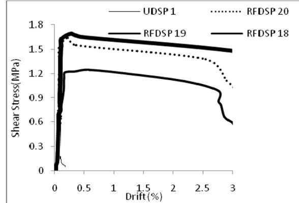
(f) Response of URM and bidirectionally retrofitted one - wythe thick masonry panel
