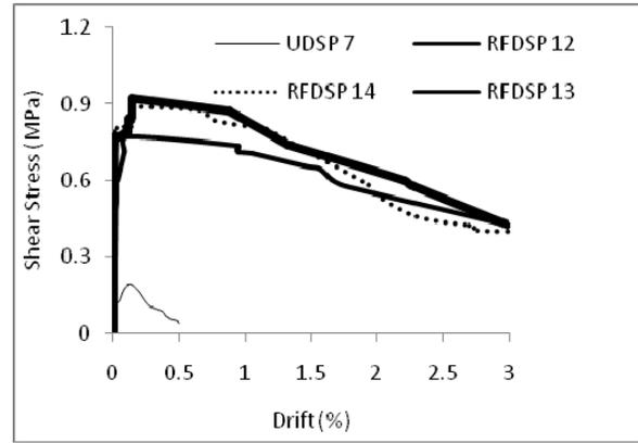
(d) Response of URM and bidirectionally retrofitted two - wythe thick masonry panel
