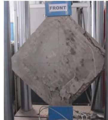
(c) Unidirectionally retrofitted two - wythe thick masonry panel
