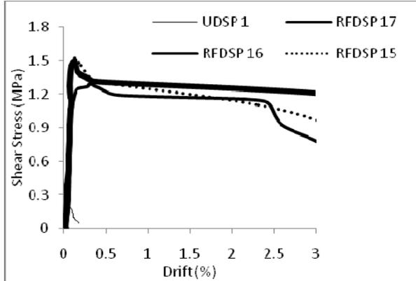
(e) Response of URM and unidirectionally retrofitted one - wythe thick masonry panel
