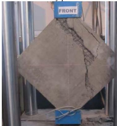
(d) Bidirectionally retrofitted two - wythe thick masonry panel
