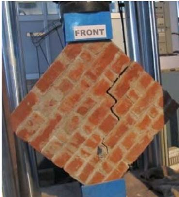
(a) URM one - wythe thick masonry panel
