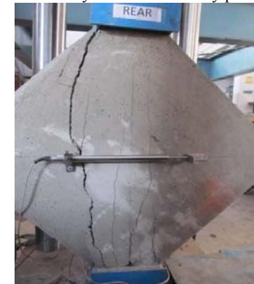
(f) Bidirectionally retrofitted one - wythe thick masonry panel
