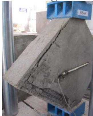
(e) Unidirectionally retrofitted one - wythe thick masonry panel
