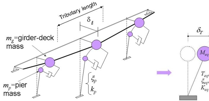
**Figure 1.** Deformation of the base-isolated bridge and equivalent SDOF model
