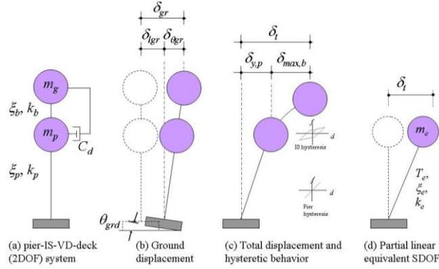
**Figure 2.** Displacements of the 2DOF and partial equivalent SDOF
