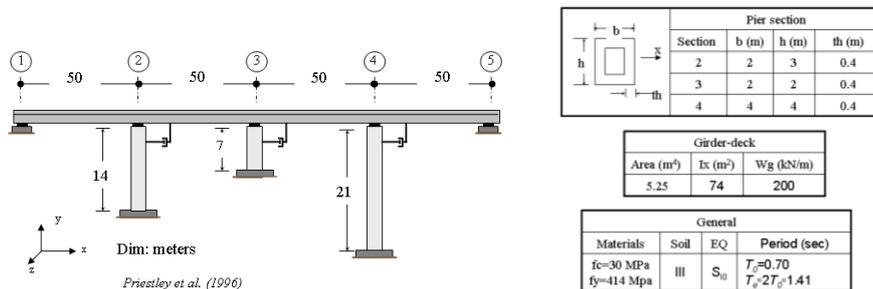
Figure 5. Geometry, properties and materials of the bridge
