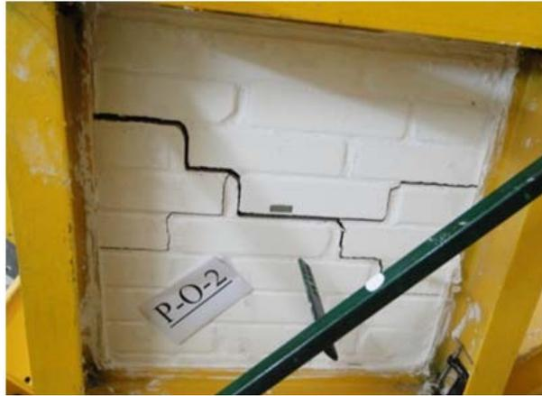
Figure 3. Out-of-plane failure of the wall panel under two-way bending
