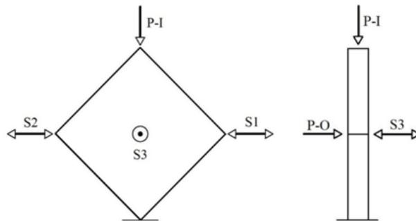
Figure 1. Position of loading jacks (P) and LVDT sensors (S) in the test set-up
