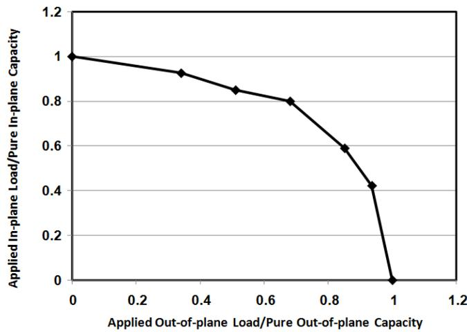
Figure 6. In-plane, out-of-plane capacity interaction curve for the wall panel
