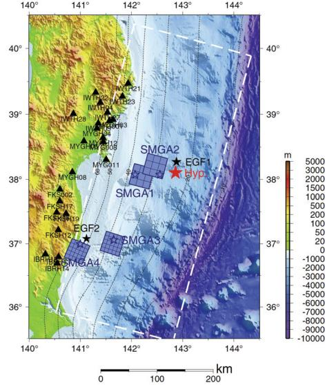
**Figure 3.2.** Map view of SMGA source model of the 2011 Tohoku earthquake
