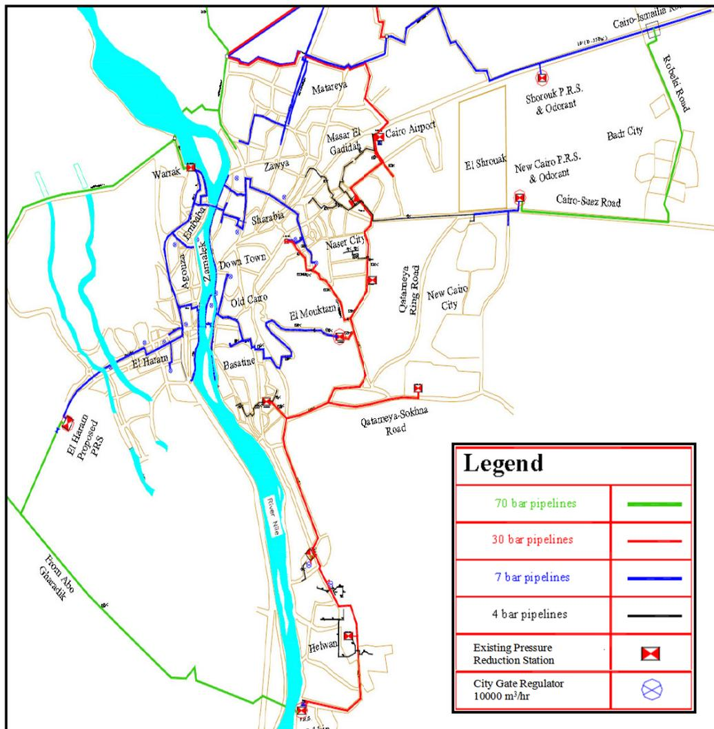
Figure 1 Greater Cairo's natural gas network, modified from EGAS (2007)
