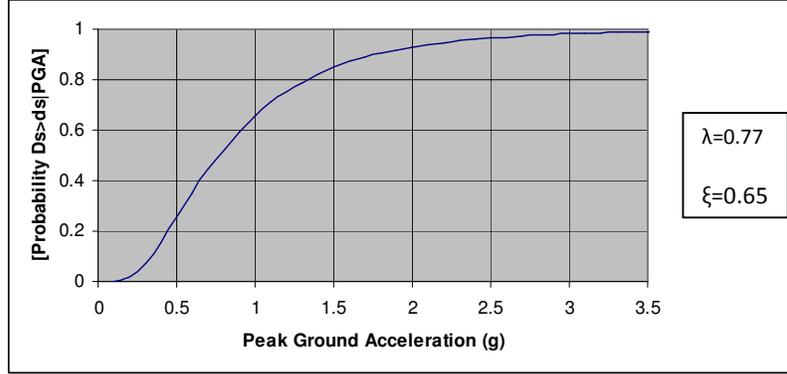
**Figure 2** Fragility curve for PRS and regulator stations,  $\lambda$  and  $\xi$  are the mean and standard deviation of the lognormal distribution respectively (Song and Ok, 2009)
