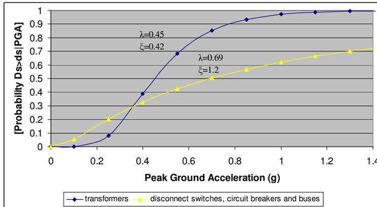
Figure 3 Fragility curves for transformers, disconnect switches, circuit breakers and buses
