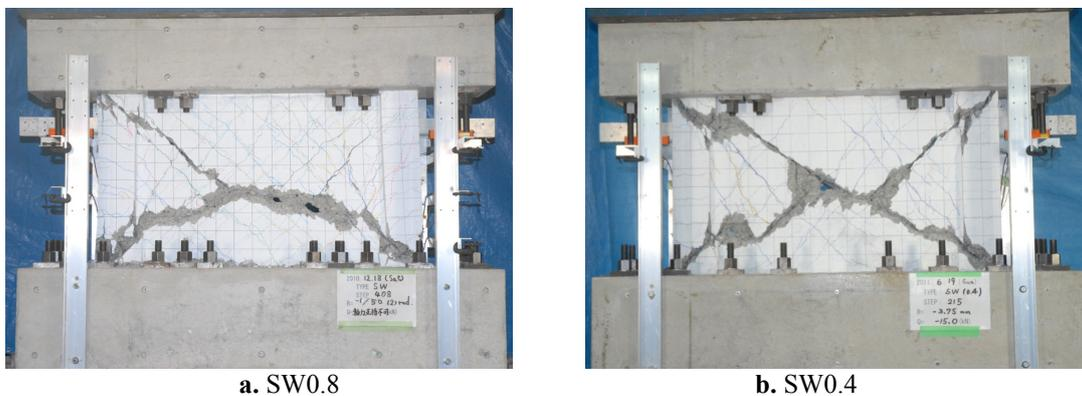
Figure 7. Damage to unstrengthened specimens after testing
