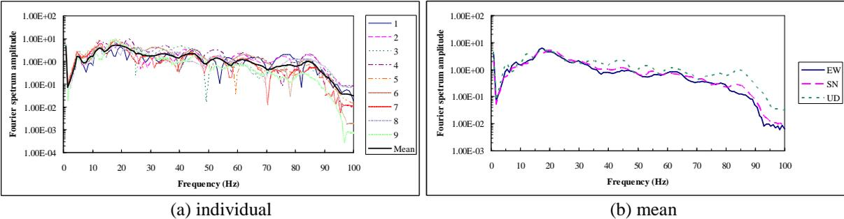
**Figure 3.4.** Frequency spectrum features of individual ground motions induced by the short delay blasting
