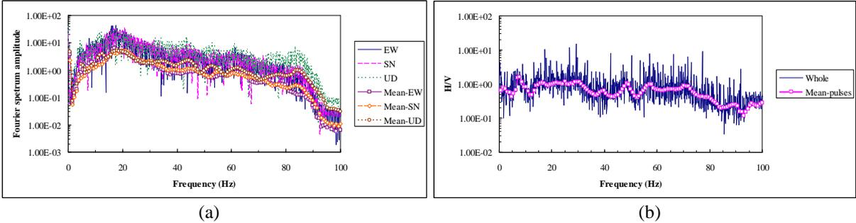
**Figure 3.5.** Difference of frequency spectrum features between whole and individual time-histories of exploding ground motion
