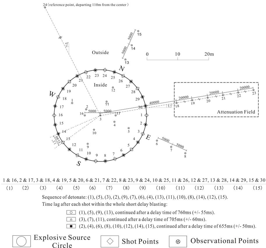
**Figure 2.1.** Design of the short delay blasting and observational points of exploding ground motion
