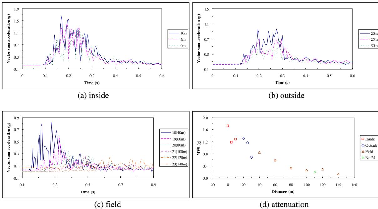
Figure 4.1. Attenuation characteristics of vibration energy induced by the short delay blasting in the target field
