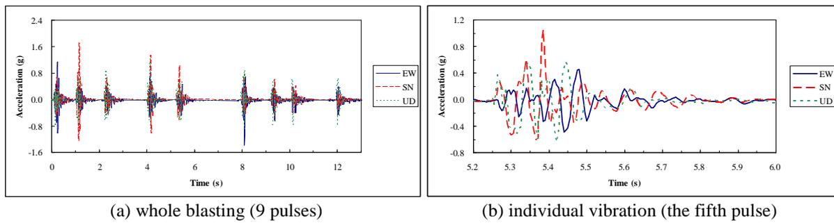
**Figure 3.1.** Time histories of strong ground motion induced by short delay blasting
