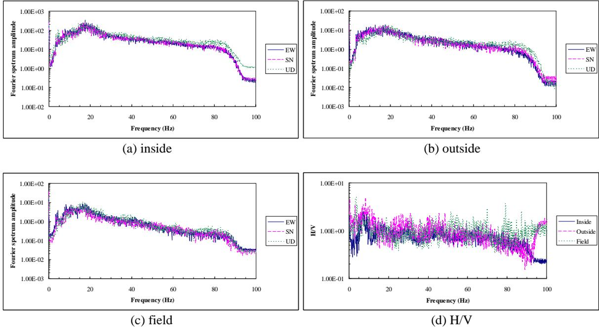
**Figure 3.6.** Different features of frequency spectrum of exploding ground motion in the target field
