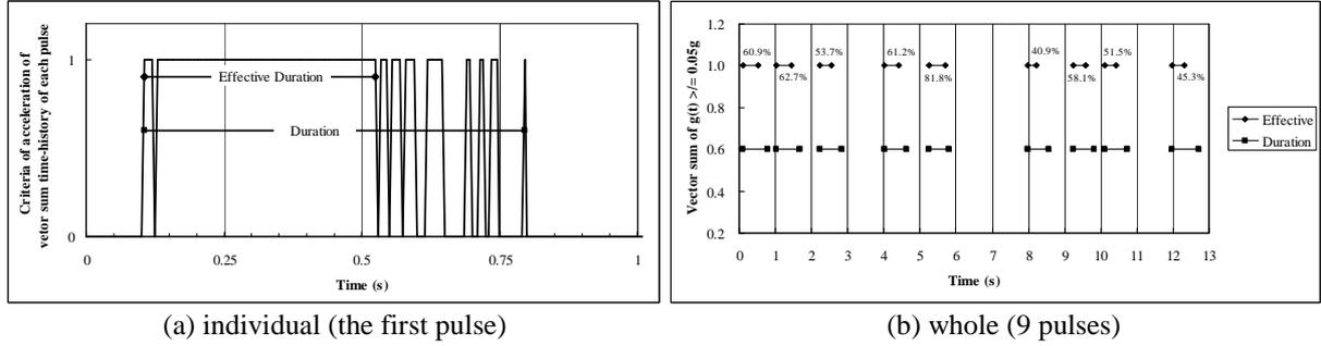
**Figure 3.2.** Duration features of recorded ground motion induced by short delay blasting
