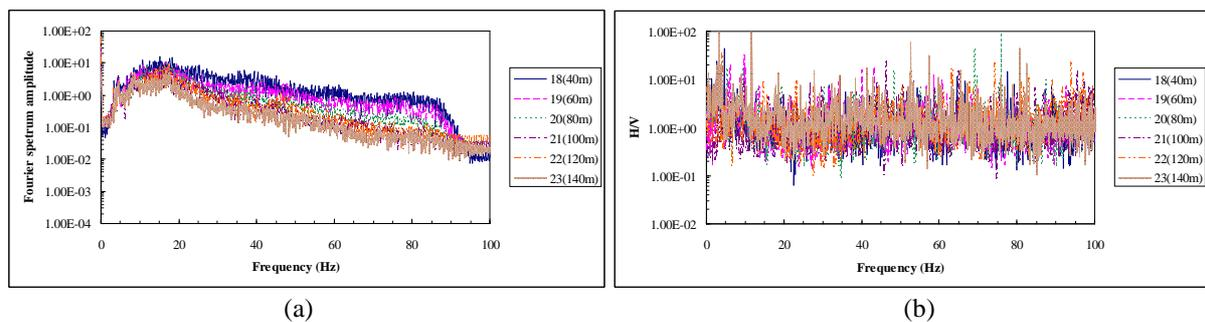
**Figure 4.2.** Attenuation characteristics of frequency spectrum of exploding ground motion
