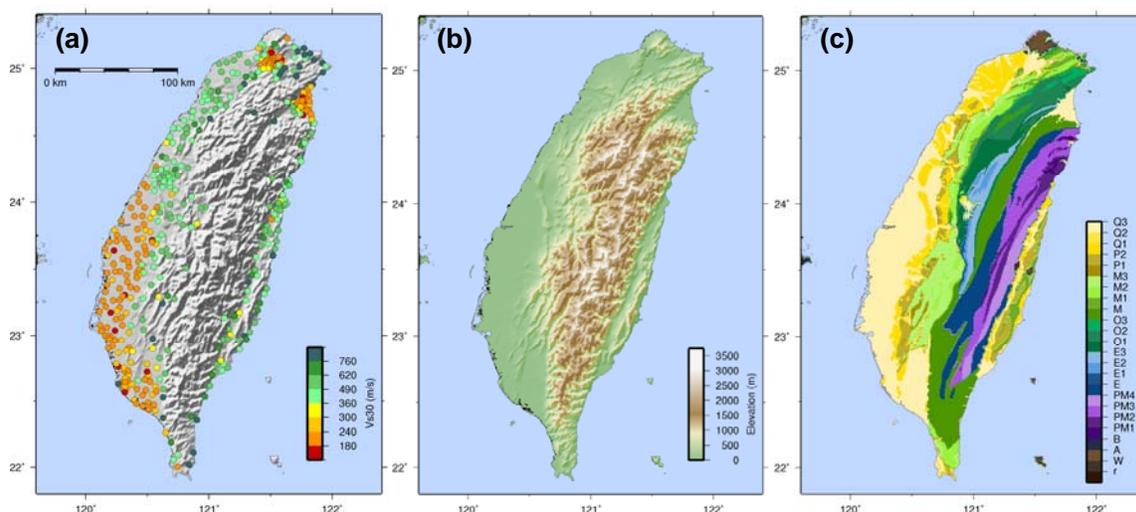
**Figure 1.** (a) NCREE  $V_{S30}$  measurements (Kuo et al., 2012). (b) SRTM 30c topography. (c) Geologic units compiled by Lee et al. (2001).
