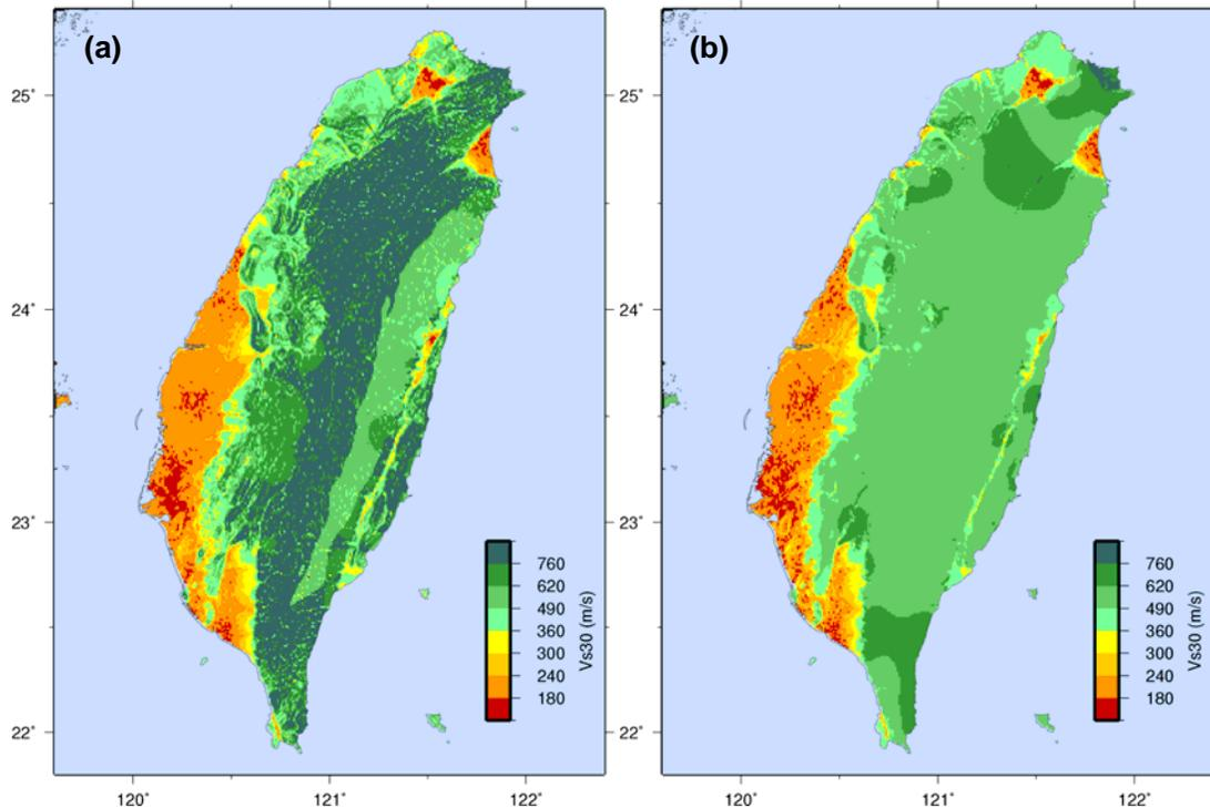
**Figure 7.** Final  $V_{S30}$  maps using the kriging-with-a-trend method where the trend is defined as a function of gradient and surface geology for (a) Strategy 1, and (b) Strategy 2.
