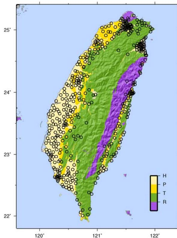
**Figure 3.** Map of the simplified geologic units summarized in Table 1. The open circles indicate the location of  $V_{S30}$  measurements.
