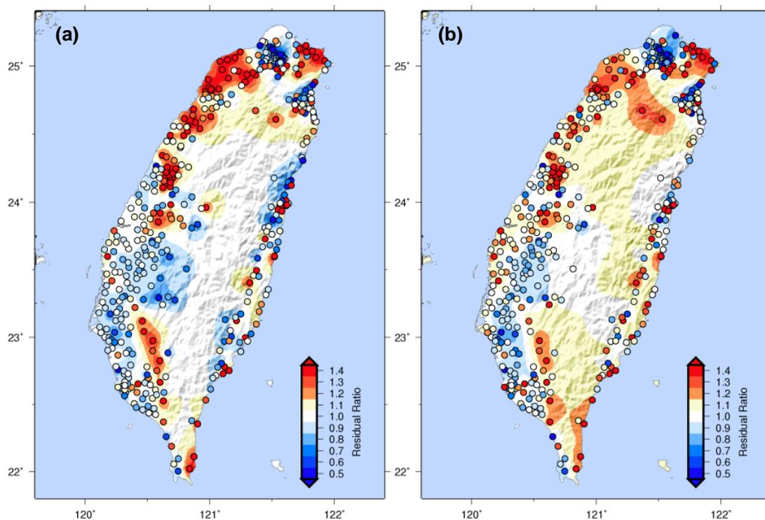
**Figure 6.** Residuals at the  $V_{S30}$  measurements and the kriged values for (a) Strategy 1 – refining the Allen and Wald (2009) approach with the Lee et al. (2001) surface geology (see Figure 4c), and (b) Strategy 2 – a separate piecewise-regression of the slope- $V_{S30}$  relationship for each geologic classification (see Figure 5).
