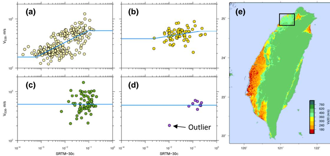
**Figure 5.**  $V_{S30}$  vs slope for (a) Holocene, (b) Pleistocene, (c) Tertiary rocks, and (d) other rock units; (e) is the map that results from applying these relationships. The outlier discussed in the text is labeled with an arrow in (d). The example region discussed in the text that is primarily Pleistocene units in (e) is labeled with a box.
