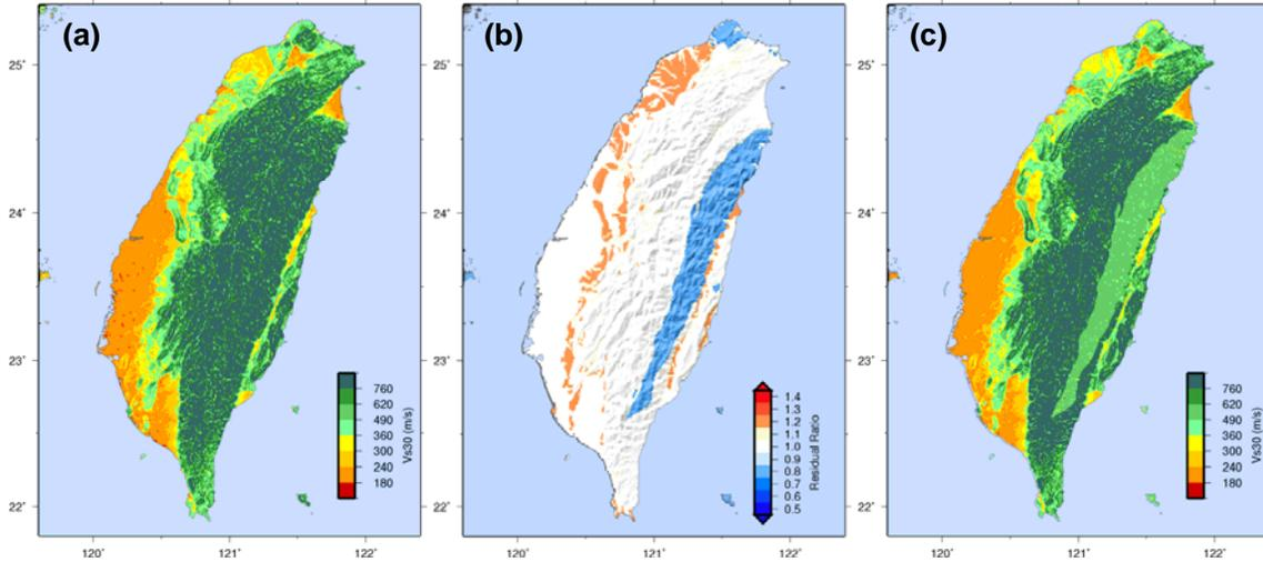
**Figure 4.** (a)  $V_{S30}$  computed with the Allen and Wald (2009) method, (b) Mean residual ratio in each the simplified geologic categories, and (c) the  $V_{S30}$  map that results from multiplying (a) and (b).
