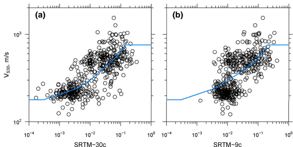
**Figure 2.**  $V_{S30}$  measurements (Kuo et al., 2012) plotted against gradients computed from (a) SRTM 30c topography, and (b) SRTM 9c topography.
