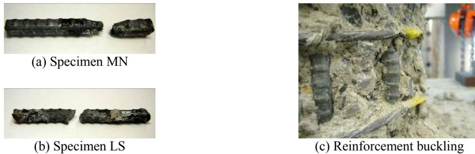
Figure 2.8. Fractured reinforcements
