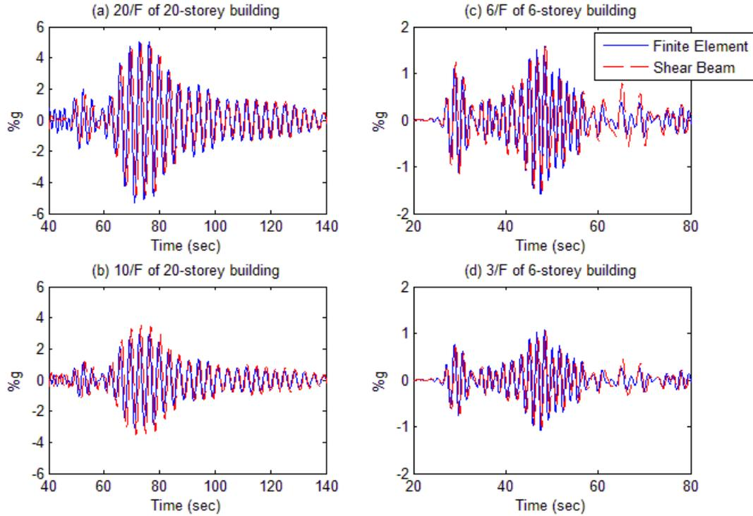
**Figure 5.** Comparison of responses from finite element models and shear beam models for the buildings in I-710/91 assuming a M 6 in San Bernadino with dip= 90°, rake= 180°, and strike = 120°. (a) Response at 20/F of 20-storey building; (b) Response at 10/F of 20-storey building; (c) Response at 6/F of 6-storey building; (d) Response at 3/F of 6-storey building
