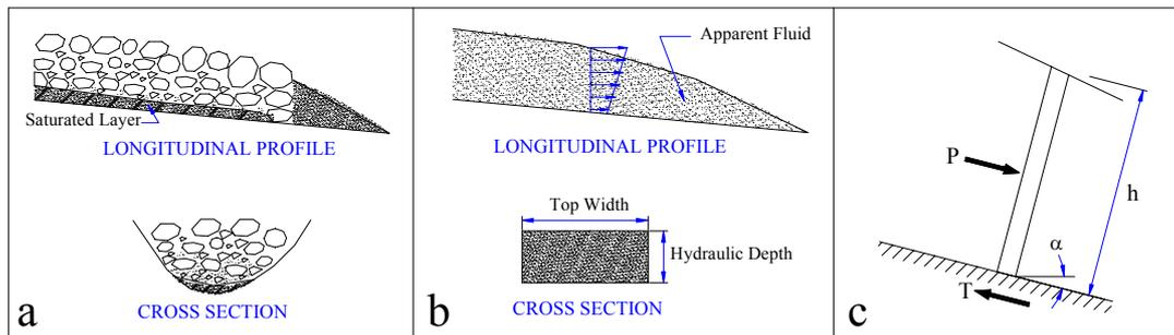
**Figure 7.** Basic concept of Depth Average Material Point Method (DAMPM) dynamic model a) prototype b) model c) forces acting on one column (after Hungr, 1995)
