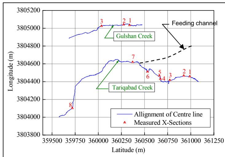
**Figure 6.** Plane profiles of Gulshan and Tariqabad creeks along with locations of cross-sectional measurements to estimate the flow velocity and discharge
