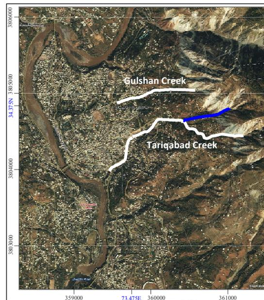
**Figure 2.** Exposed debris source behind Muzaffarabad city and incised creeks feeding Neelum River (Modified from IKONOS © SPACEIMAGING 2005)
