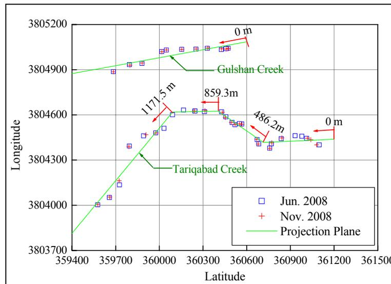
**Figure 3.** Marked data points along Gulshan and Tariqabad creeks along with common projection planes (with UTM coordinates)
