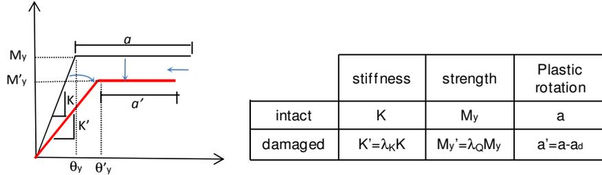
**Figure 2.** Modeling criteria for the damaged plastic hinges (adapted from (FEMA, 1998a))
