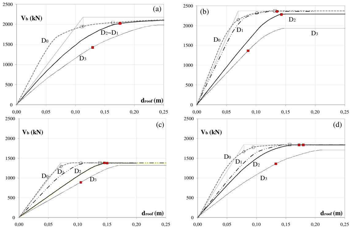
**Figure 3.** Pushover curves for the building in the three considered damage configurations ( $D_{1,2,3}$ ) and for the intact structure ( $D_0$ ): cases MAX (a), MAY (b), MOX (c) and MOY (d).
