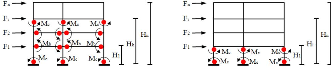
**Figure 5.** Example of collapse mechanism types.
