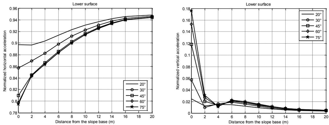
**Figure 3.3.** Normalized acceleration response horizontal (a) and vertical (b) on the lower surface
