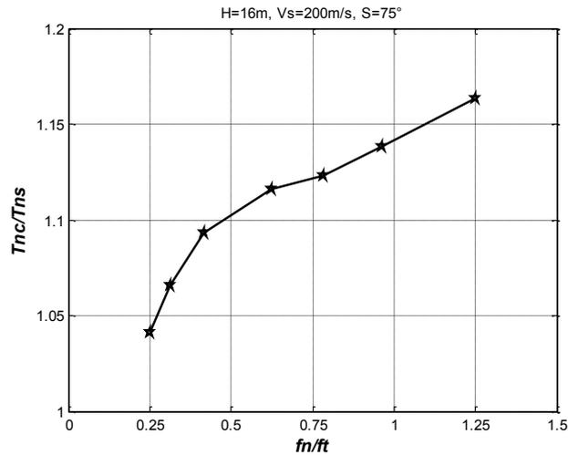
**Figure 5.3.** Variation of the of peak amplification ratios  $T_{nc}/T_{ns}$  with  $f_n/f_t$
