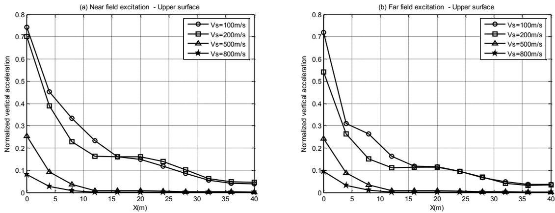
Figure 4.2. Normalized vertical acceleration response to near field excitation (a) and far field excitation (b)
