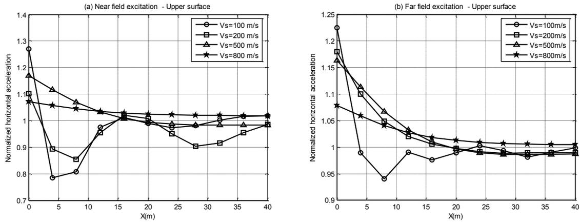
Figure 4.1. Normalized horizontal acceleration response to near field excitation (a) and far field excitation (b)
