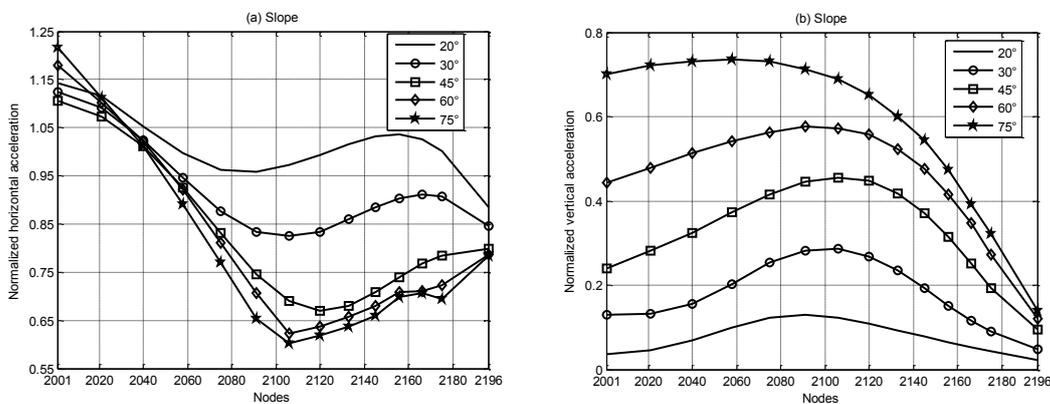
Figure 3.2. Normalized acceleration response horizontal (a) and vertical (b) on the slope
