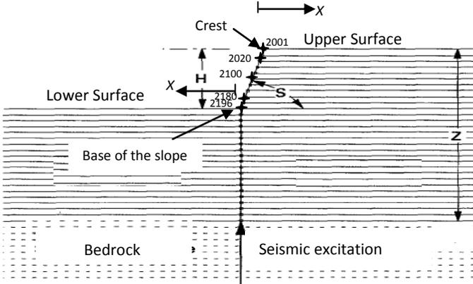
**Figure 2.1.** Configuration of the slope
