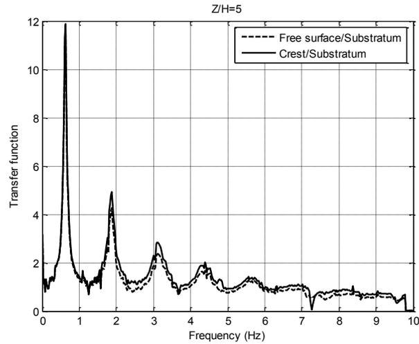
**Figure 5.2.** Transfer functions (free surface/Substratum, Crest/Substratum) for  $\frac{Z}{H} = 5$
