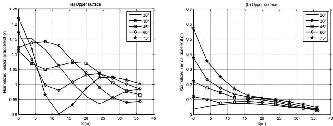
Figure 3.1. Normalized acceleration response horizontal (a) and vertical (b) on the upper surface
