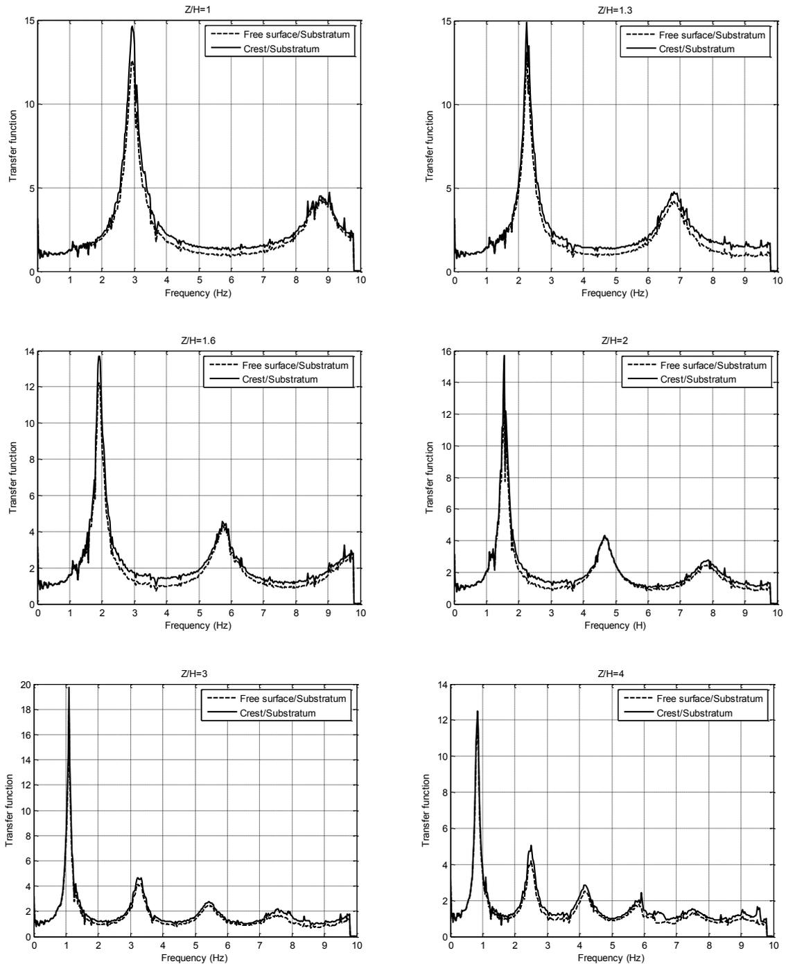
**Figure 5.1.** Transfer functions (free surface/Substratum, Crest/Substratum) for different ratios  $Z/H$
