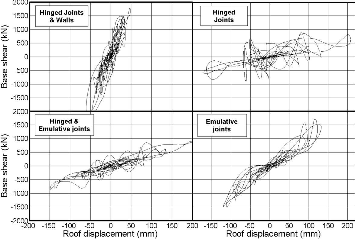
Figure 5. Base shear versus roof displacement response of the four structural systems at PGA of 0.30g.
