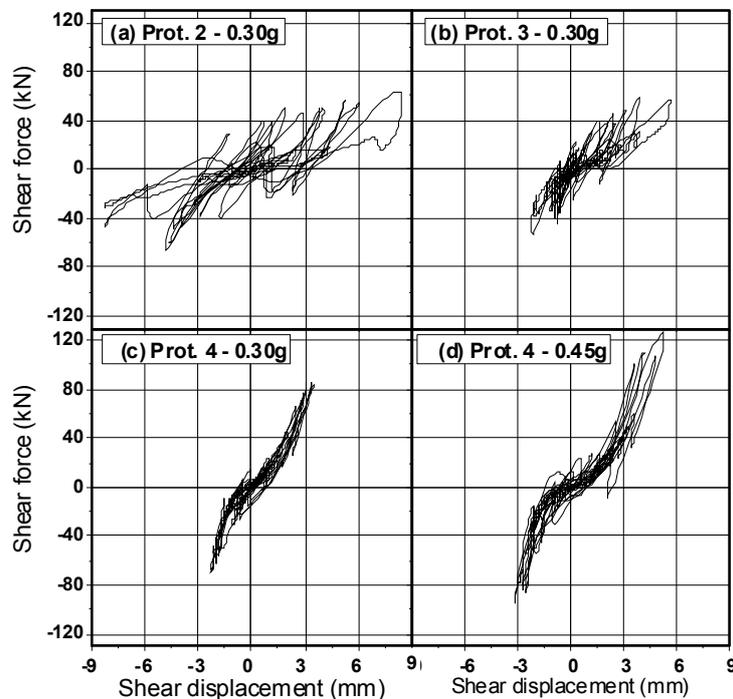
**Figure 6.** Joint shear force versus the joint slip loops for a beam-column joint of the third floor of: (a) Prototype 2 at PGA 0.30g. (b) Prototype 3 at PGA 0.30g. (c) Prototype 4 at PGA 0.30g. (d) Prototype 4 at PGA 0.45g.
