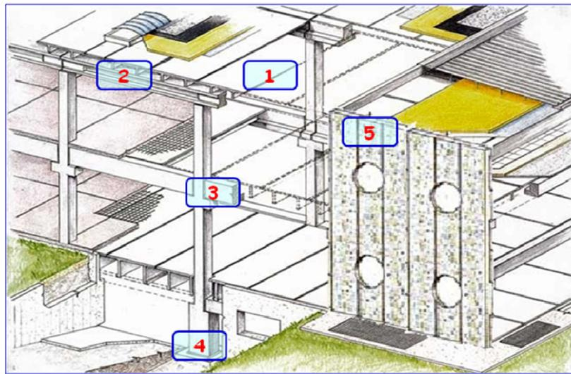
**Figure 1.** Categories of connections between the different structural elements of a precast concrete building.
