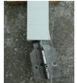
(a) Buckling (b) Buckling Zone Figure 3.10. MRL1.0S2 Collapse Mode
