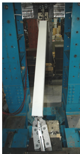
Figure 1.1. Overall Buckling of BRB including connections
