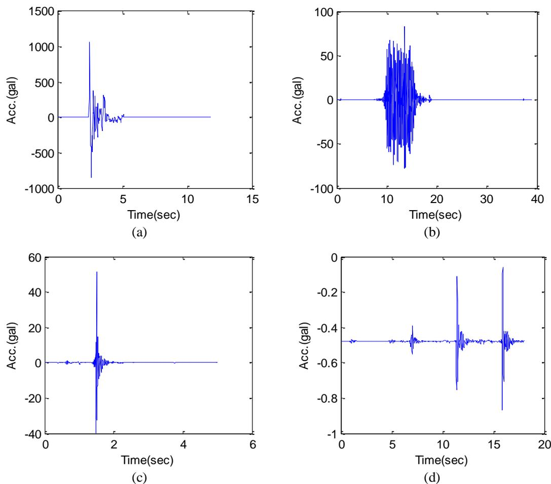
**Figure 1.** wave form of four kinds of typical noise: a, quarry blasts; b, high speed train; c, heavy machinery; d, thunder storm
