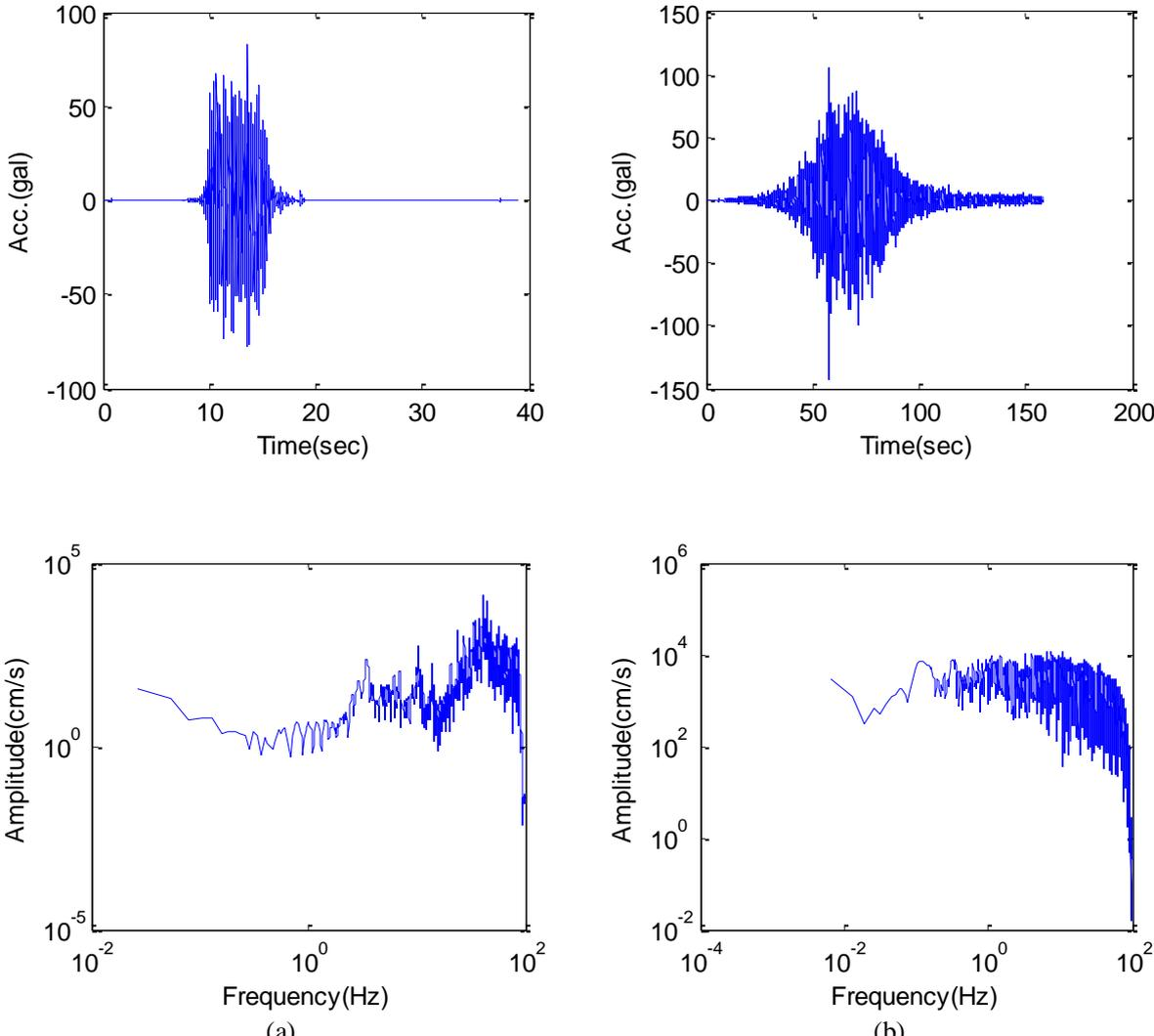
**Figure 4** Frequency spectra of train noise(a) and earthquake(b)
