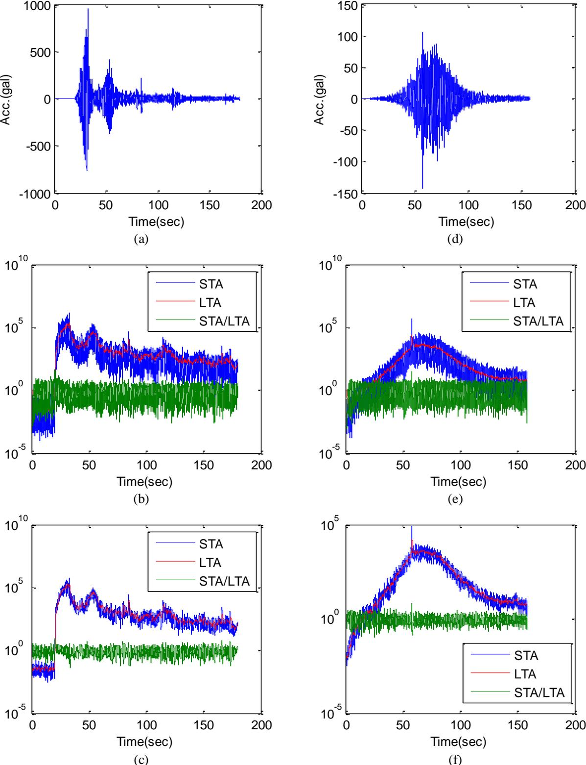
**Figure 2.** (a) is EW component in WCW station from WenChuan earthquake; (b) STA/LTA of WCW according to equation (1.2); (c) STA/LTA of WCW according to equation (1.3); (d) is EW component in WIX station from WenChuan earthquake. (e) STA/LTA of WIX according to equation (1.2); (f) STA/LTA of WIX according to equation (1.3); Long window is 1 second and short window is 0.1 second.
