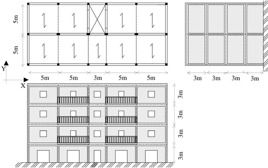
Figure 1. Typical layout of the examined RC frame buildings
