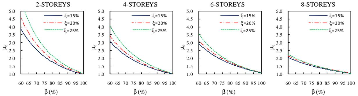
**Figure 9.** Average ductility demand ( $\mu_d$ ) as a function of the strength reduction factor ( $\beta$ ) imposed to the superstructure ( $\alpha=10\%$ ,  $r_s=3\%$ ) of 2-, 4-, 6- and 8-storeys buildings equipped with LRB at 0.5g PGA
