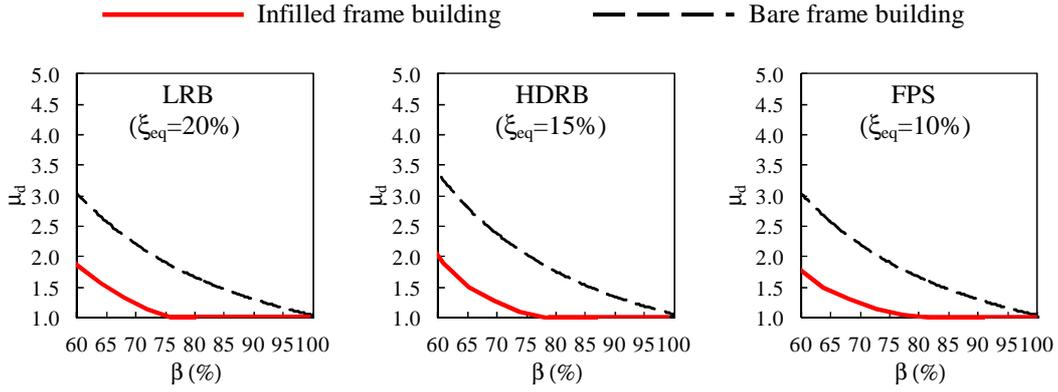
**Figure 11.** Effects of masonry infills on the ductility demand to the superstructure of a 4-storeys building ( $\alpha = 10\%$ ), equipped with different types of isolation system at 0.5g PGA
