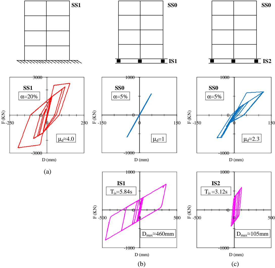
**Figure 5.** Different strategies in the seismic protection of a 4-storeys building with  $\alpha=5\%$ : (a) lateral strengthening, (b) use of an isolation system ( $\xi \approx 25\%$ ) designed to prevent yielding in the superstructure, (c) use of an isolation system designed to limit the maximum base displacement while accepting a ductility demand of 2 in the superstructure.
