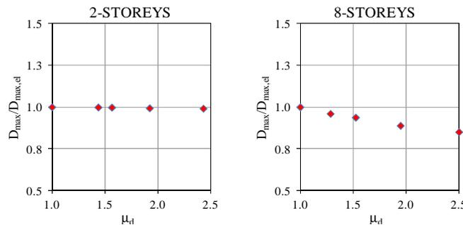
**Figure 8.** Changes in the maximum displacement response of the isolation system due to the hysteretic cyclic behavior of the superstructure, for different values of ductility demand
