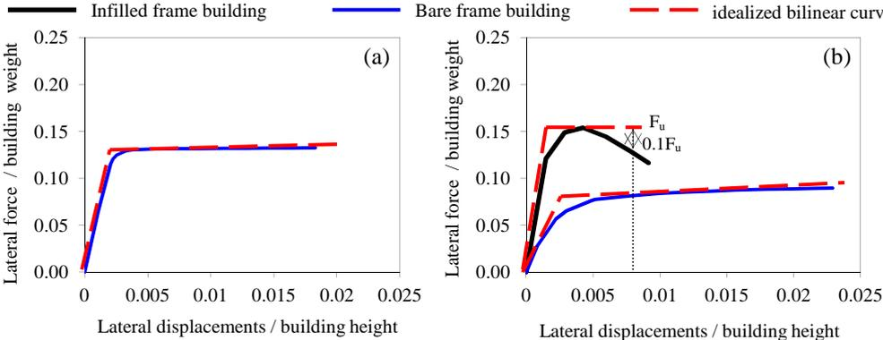
Figure 2. Typical pushover curves of the examined RC frame buildings in their (a) strong and (b) weak direction
