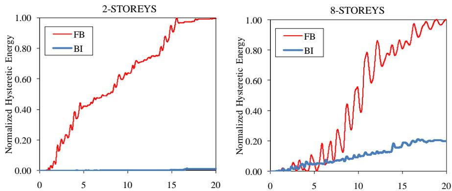
**Figure 7.** Comparison between the hysteretic energy dissipated by the superstructures of Fixed-Base (FB) and Base-Isolated (BI) buildings experiencing similar ductility demands under the same earthquake.
