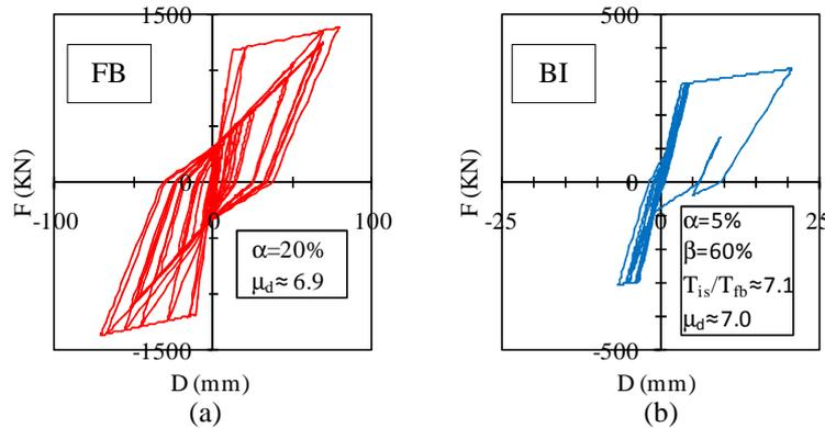
**Figure 6.** Comparison between the cyclic hysteretic behaviors of the superstructures of 2-storey (a) fixed-base and (b) base-isolated buildings experiencing similar ductility demands.
