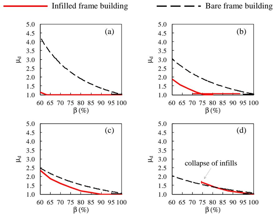
**Figure 12.** Effects of masonry infills on the global ductility demand to the superstructure of (a) 2-, (b) 4-, (c) 6- and (d) 8-storeys BI-buildings equipped with LRB ( $\xi_{eq} \approx 20\%$ ), at 0.5g PGA.
