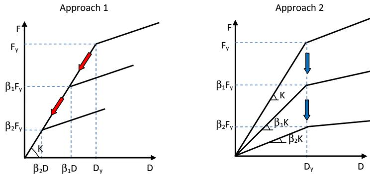
**Figure 3.** Different approaches followed in the reduction of the lateral strength of the superstructure
