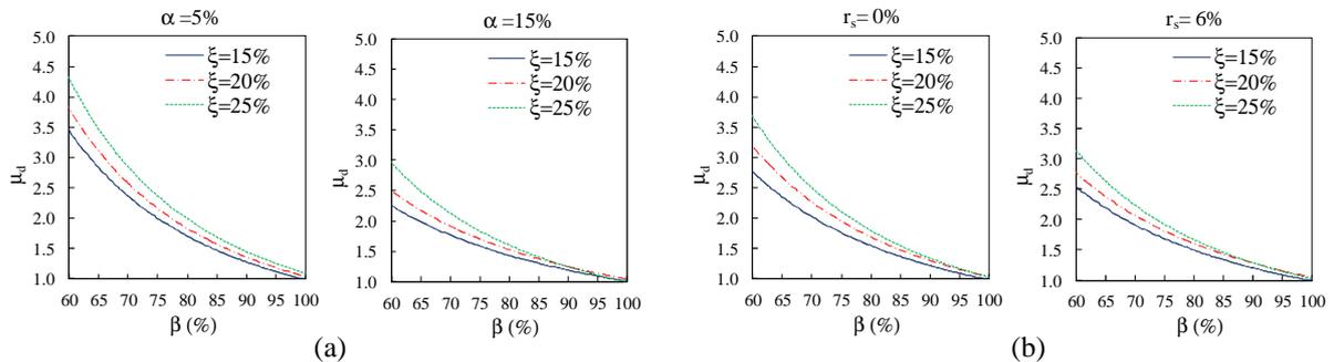
**Figure 10.** Effects of (a) strength ratio ( $\alpha$ ) and (b) post-yield stiffness ratio ( $r_s$ ) on the global ductility demand to the superstructure ( $\mu_d$ ) of a 4-storeys base-isolated (LRB) building, at 0.35g PGA
