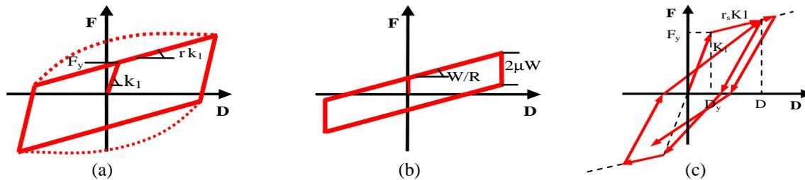
Figure 4. Idealized cyclic behavior of (a) LRB-HDRB, (b) FPS and (c) RC building.
