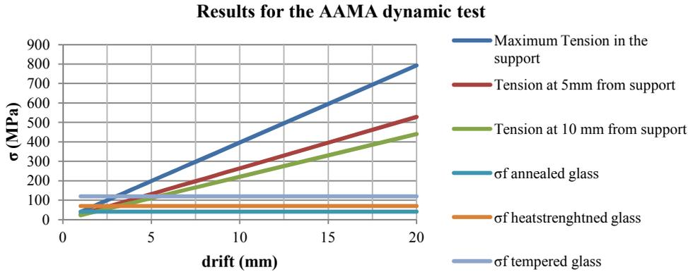
Figure 4.6. An example of the results obtained for the dynamic crescendo test.
