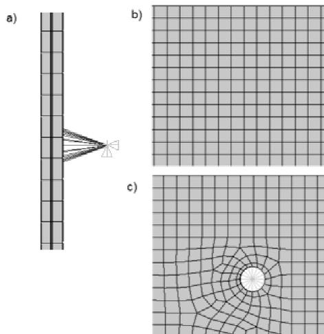
**Figure 4.2.** FE mesh details - a) lateral view; b) interior of the panel; c) support region.
