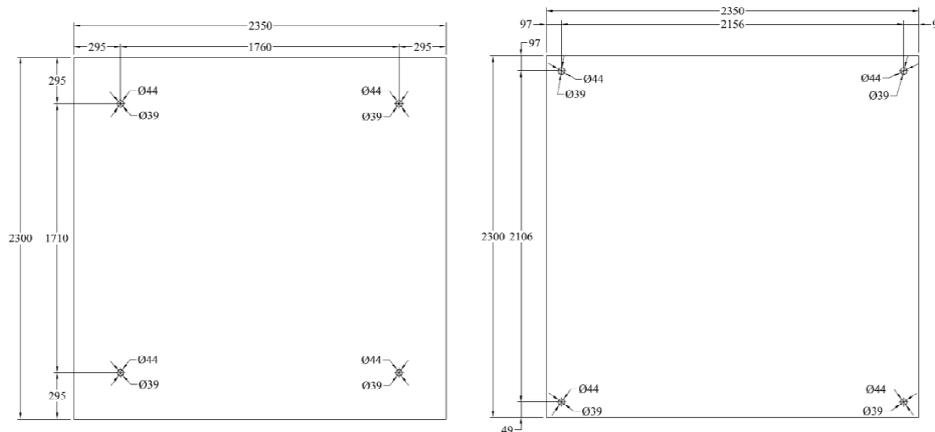
Figure 4.1. Geometrical configuration of the glass panels: Left) V1 and V2; Right) V3, V4 and V5.
