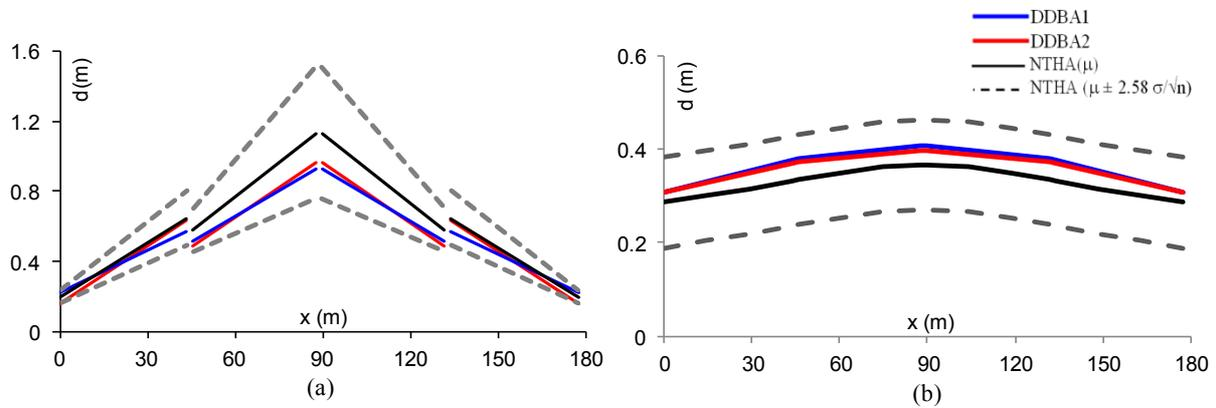
**Figure 5.** Comparison between DDBA predictions and NTHA results ( $\mu \pm 2.58 \sigma/\sqrt{n}$ ) in terms of maximum deck displacements associated to the DS2 in the transverse direction of the bridge with (a) independent decks and (b) continuous deck.
