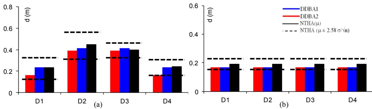
**Figure 6.** Comparison between DDBA predictions and NTHA results ( $\mu \pm 2.58 \sigma/\sqrt{n}$ ) in terms of maximum deck displacements associated to the DS2 in the longitudinal direction of the bridge with (a) independent decks and (b) continuous deck.
