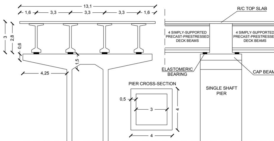
Figure 1. Structural scheme of the selected case study.
