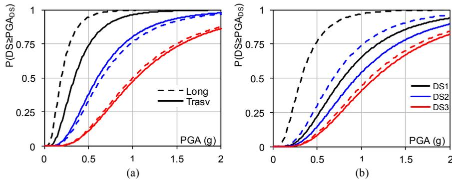
**Figure 3.** Fragility curves of the selected bridge with (a) continuous deck and (b) independent spans.
