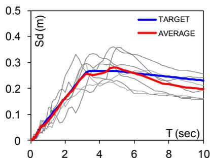
**Figure 4.** 5%-damped displacement response spectra of the accelerograms used in the NTHA.
