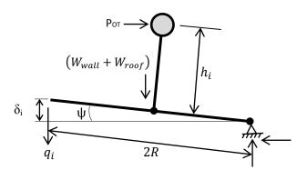
Figure 5. Simplified model undergoing rocking.
