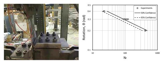
Figure 2. Shell-base connection test (left); rotation vs. number of cycles to failure curve (RN curve) (right).
