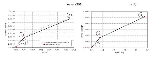
Figure 4. Moment vs. base rotation curve (left); force vs. uplift displacement curve for the spring (right).
