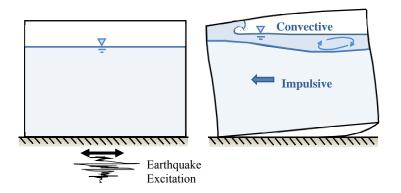
Figure 1. Tank at rest (left); uplifted tank showing the impulsive and convective liquid masses (right).
