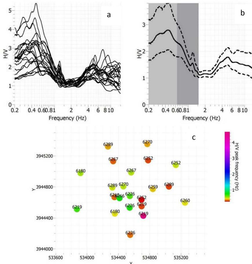
Figure 3: a) H/V curve for 22 stations. b) Mean value of H/V c) H/V peak frequency for each station
