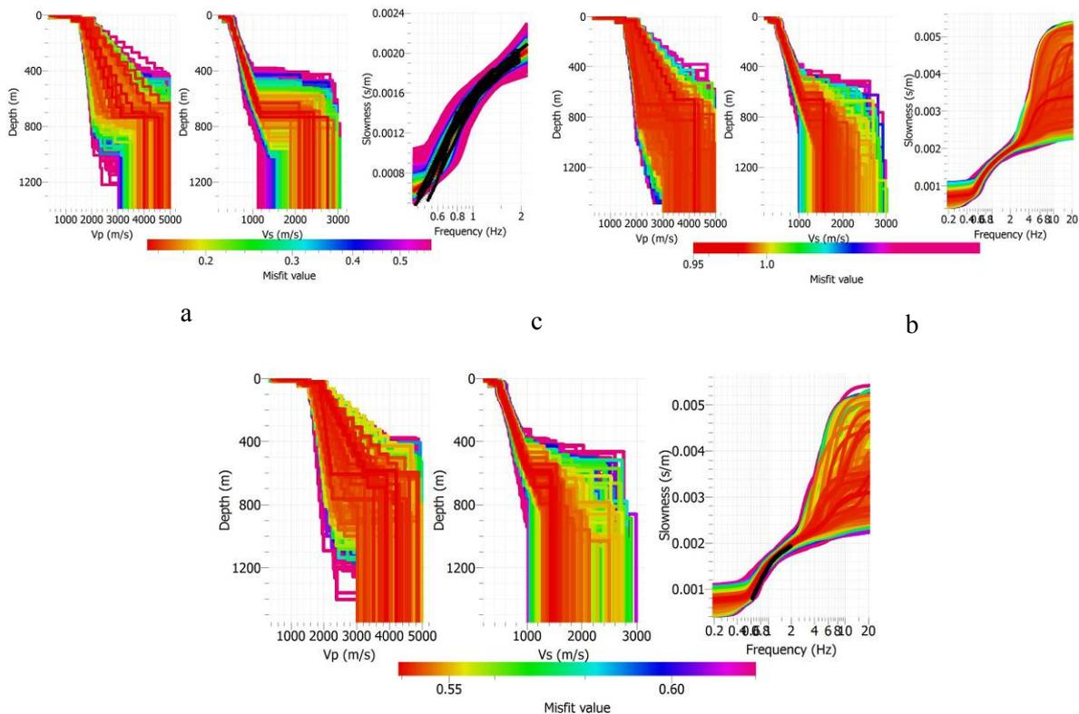
Figure 7 : Dispersion curve and ground profile to 1500 m. a)F-K b)SPAC c) joint inversion of F-K and SPAC
