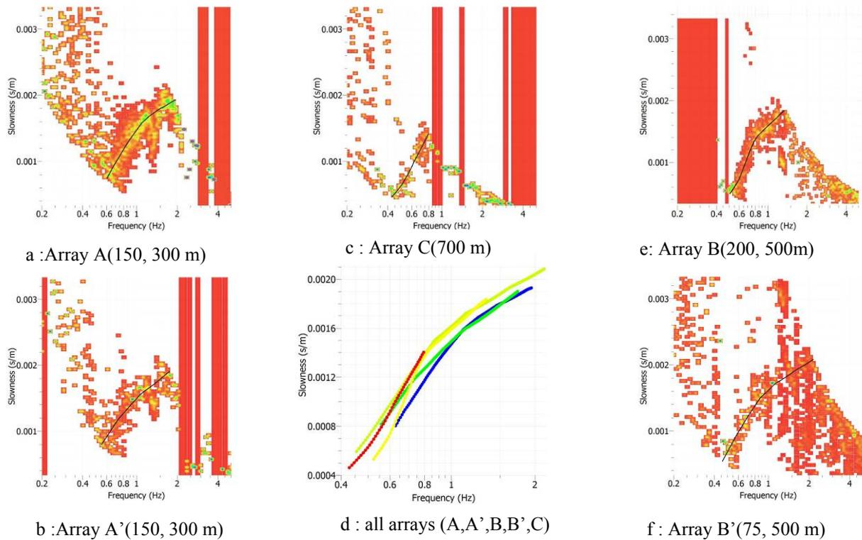
Figure 4 : F-K analysis dispersion curves for all arrays. This figure shows slowness against frequency for windows having semblance and beam power greater than 70%. All the dispersion curves were plotted together in panel d (blue: array A; green: array A'; yellow: Array B, olive: Array B' and red: array C)
