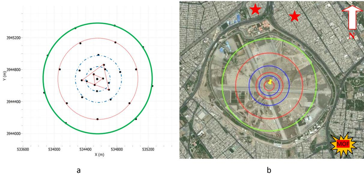
Figure 2: a) stations design in five arrays, (array A, A' : blue dashed line, array B,B' : red dotted line and Array C : green line) b) satellite image over Gale Morghi site (blue circle and red stars shows geotechnical site investigations and location of Downhole test consecutively)
