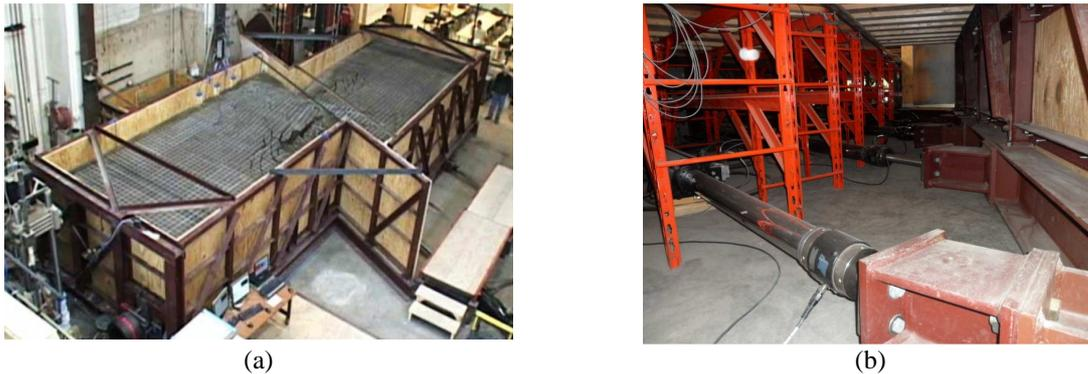
**Figure 1** Large scale soil-pipeline test at Cornell University: (a) large-scale experiment; (b) hydraulic structural actuators.
