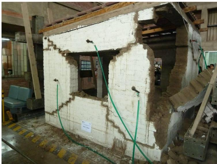
**Figure 12.** View on collapsed wall of module after test
