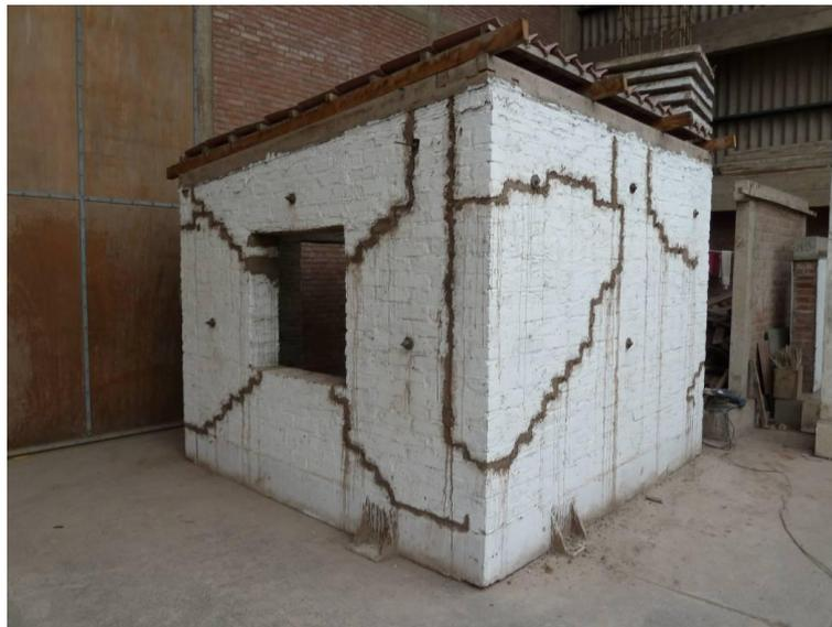
**Figure 10.** Adobe model with all major seismic cracks repaired
