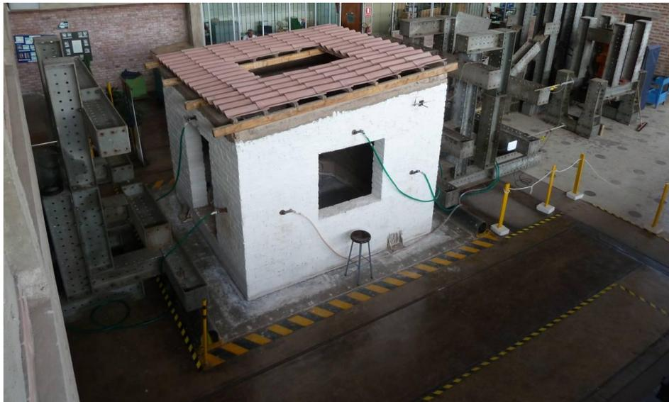
**Figure 5.** Full-scale model on shaking table
