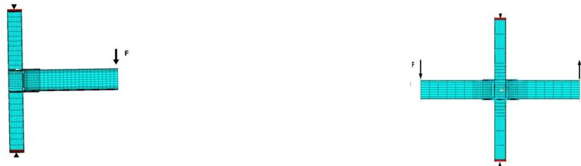
Figure 2.4. The connection subassembly was used in the finite element study.
