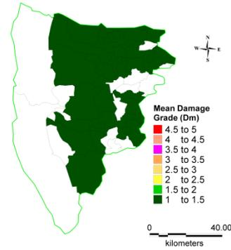
**Figure 4.4.** Mean Damage Grade ( $D_m$ ) for an assumed  $I_0=XI$  2008 Baluchistan earthquake
