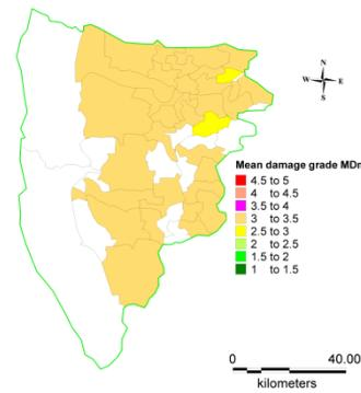
**Figure 4.8.** Damage scenario for 1 m flood height
