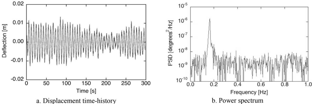
Figure 8. Measurements at level 54 of the Sky Tower.
