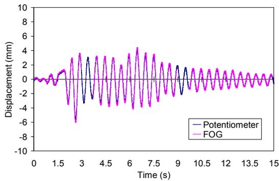
c. Relative displacement at first floor
