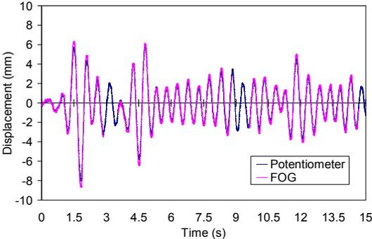
c. Relative displacement at first floor
