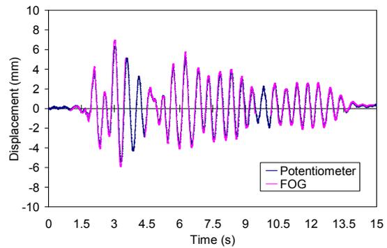
c. Relative displacement at first floor
