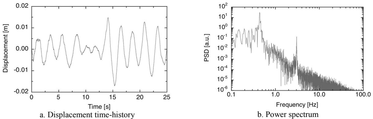
**Figure 9.** Measurements at the wind generator (turn off).
