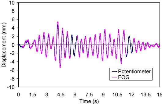
c. Relative displacement at first floor
