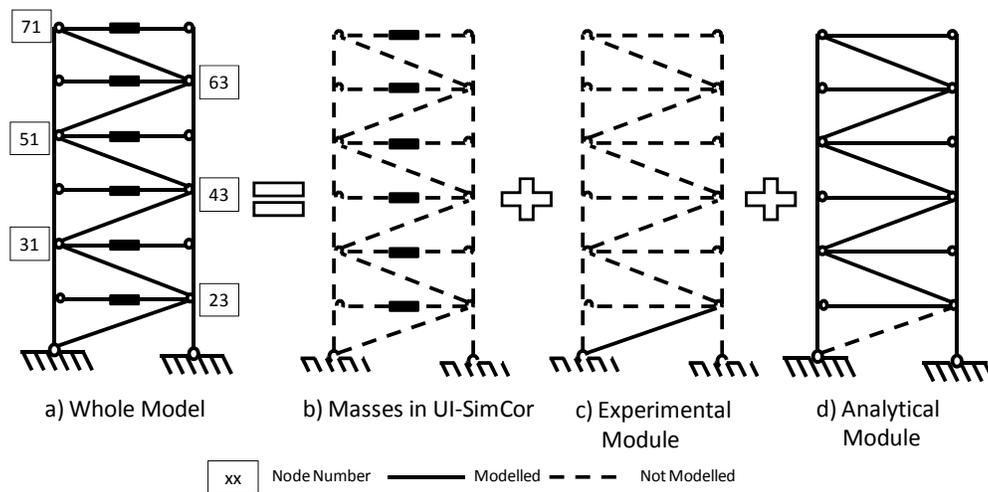
**Figure 4.** Hybrid Model with the different components
