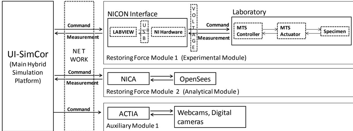
Figure 5. Communication flow among components of the hybrid simulation framework
