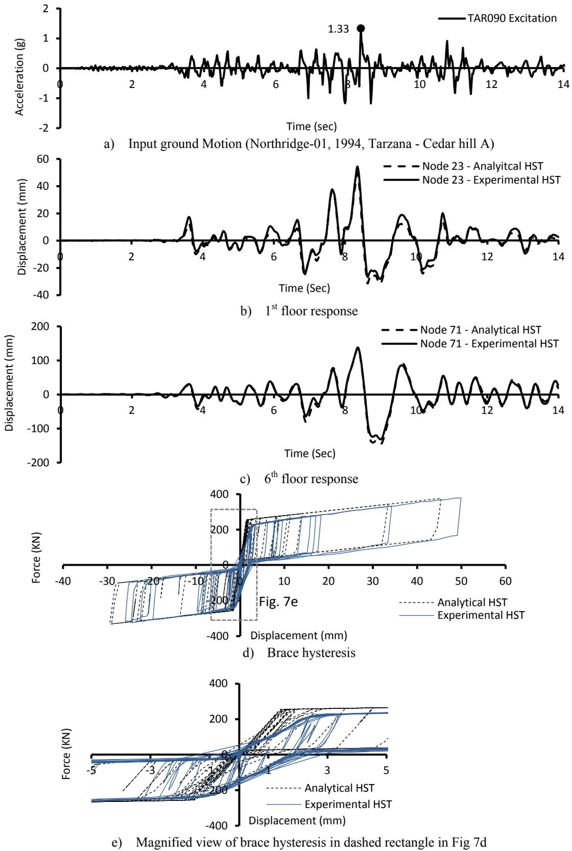
**Figure 7.** Comparison of responses from hybrid simulation and analytical prediction
