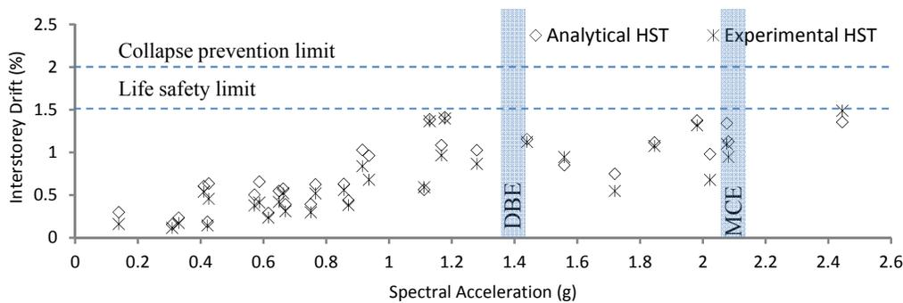
**Figure 9.** Graph showing the variation of interstorey drift with spectral acceleration
