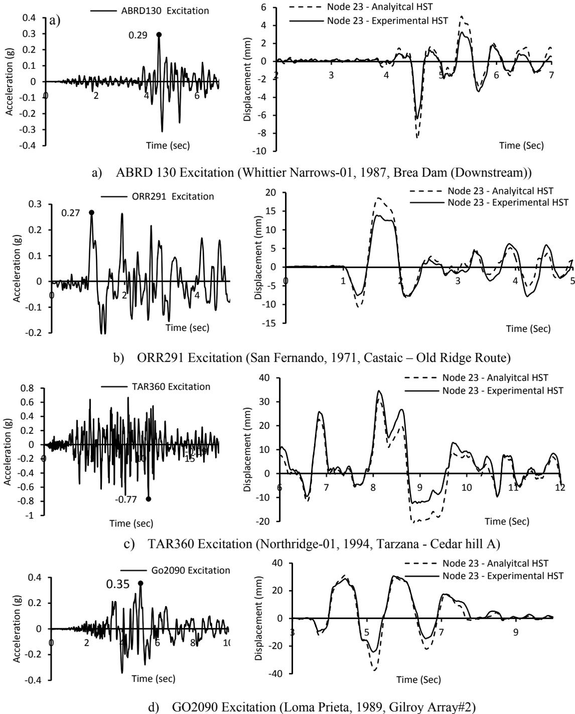
**Figure 8.** Comparison of dynamic analysis for different ground excitations; earthquake name, year and recorded station are shown in the brackets.
