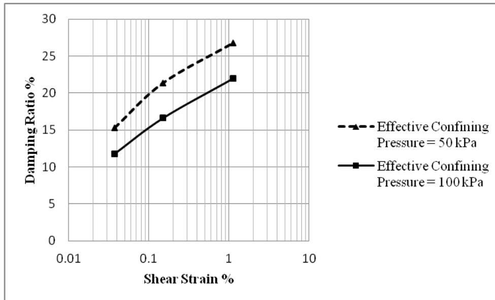
**Figure 6.2.** Influence of eff. confining press. on damping ratio versus shear strain at 0.25 % coir fiber
