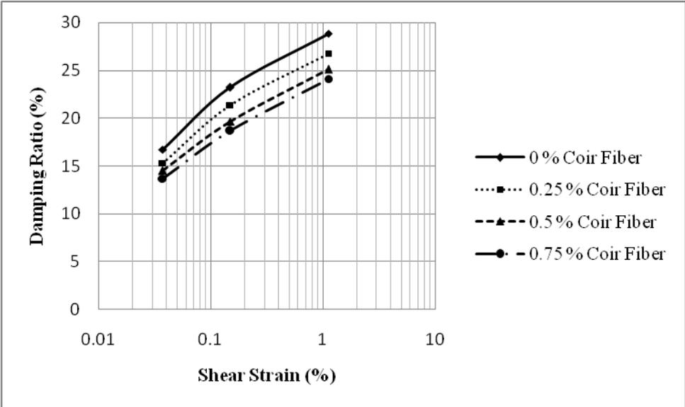
**Figure 5.4.** Influence of fiber content on damping ratio versus shear strain
