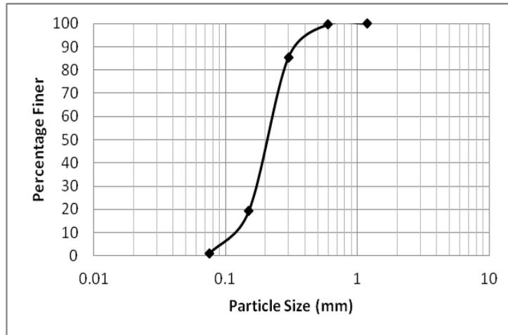
**Figure 2.1.** Grain size distribution for Solani sand
