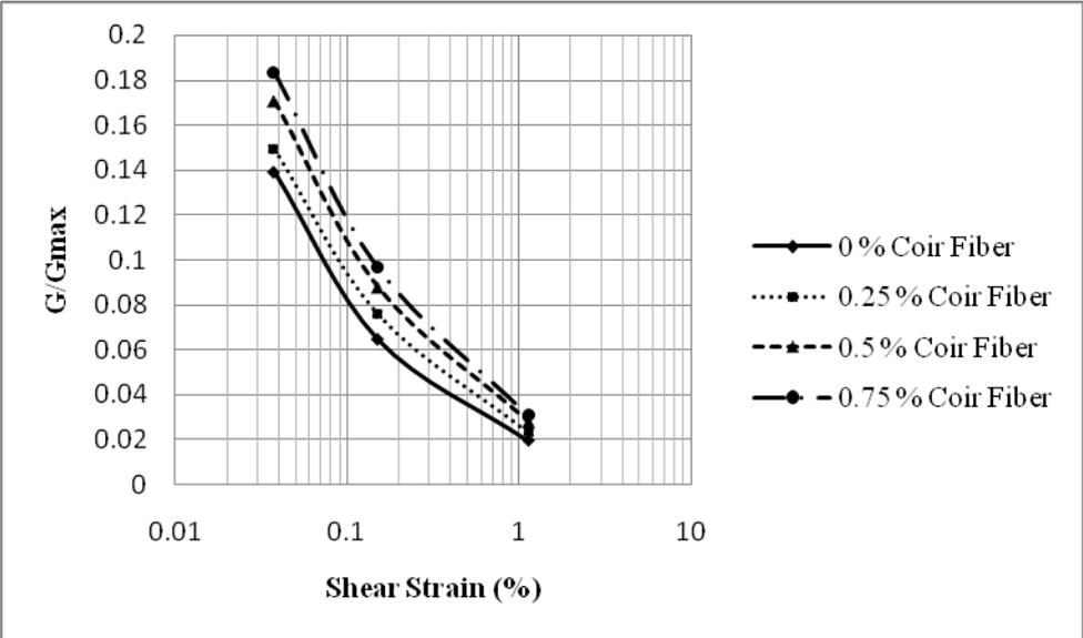
**Figure 5.3.** Influence of fiber content on normalized shear modulus versus shear strain
