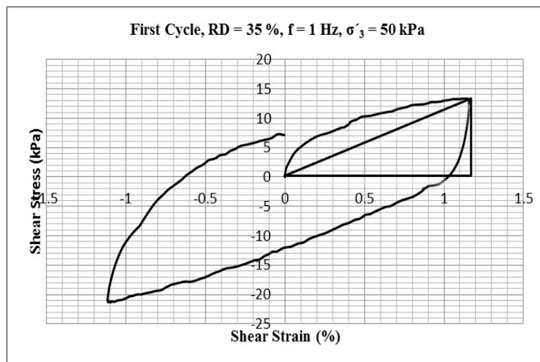
**Figure 5.2.** Shear stress vs. shear strain at first cycle for sand with 0.25% coir fiber at 1.125% shear strain
