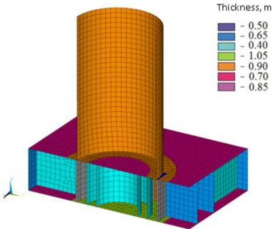
Figure 6. 3D fragment of the shaft model
