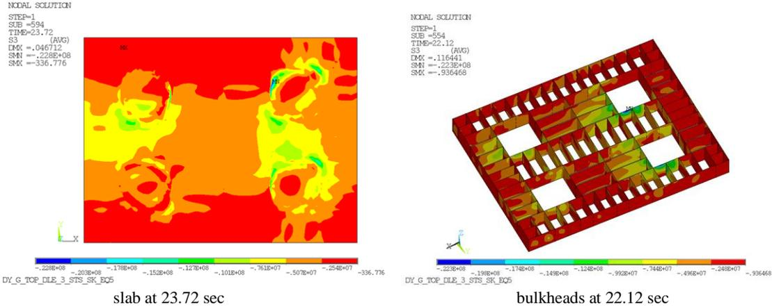
**Figure 9.** Minimum main stresses  $\sigma_3$  under seismic impact of DLE level (Pa)
