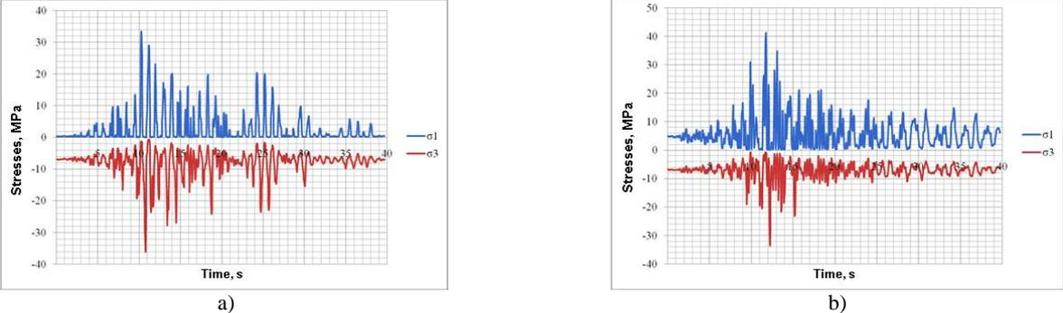
**Figure 8.** Maximum tension in the shaft ( $\sigma_1$ ) and accompanying compression ( $\sigma_3$ )
